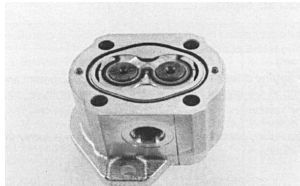
13. Gently slide the gear housing over the rear bearing block assembly, slide housing down until the housing engages the dowel pins. Press firmly in place with hands, do not force or use any tool. Check to make sure the in-take port in the housing is on the same side as the open end of the E-seal and that the marked lines on the mounting flange and gear housing are in alignment.
