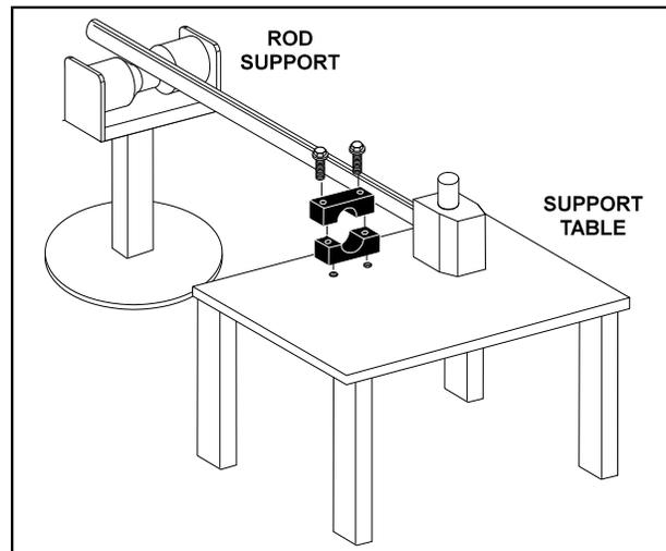
Figure 5-63. Cylinder Rod Support
