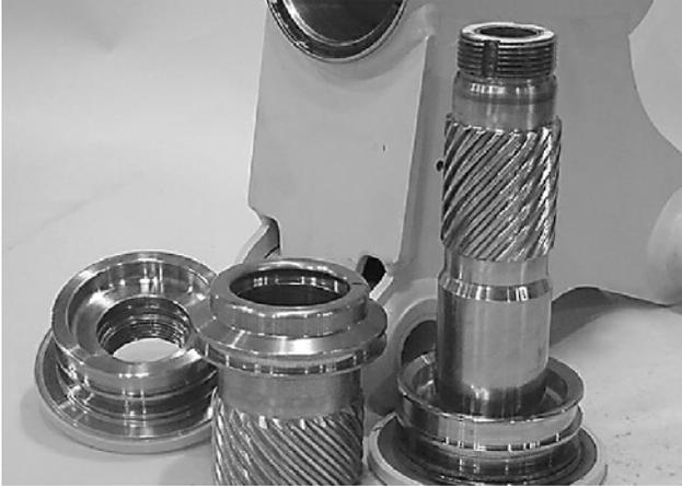
2. Inspect thrust washers (304) for rough or worn edges and surfaces. Measure thickness to make sure it is within specifications (Not less than 0.092" or 2.34 mm).
