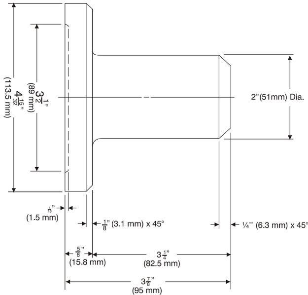
2. T-138903 ASSEMBLY PRESSING TOOL for CUP (1C)
