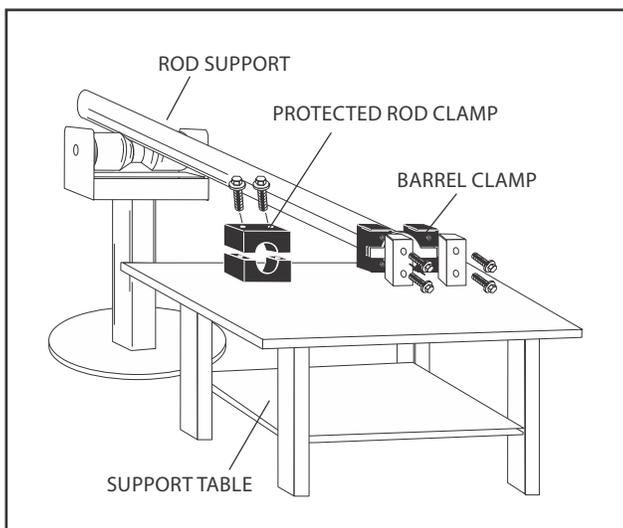
Figure 5-41. Cylinder Barrel Support
