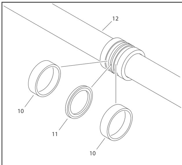
**Figure 5-65. Piston Seal and Wear Ring**
