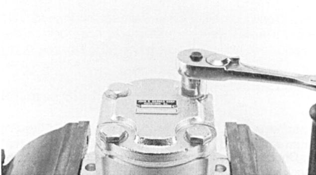
5. Clamp the mounting flange in a protected jaw vise with the pump shaft facing down.
