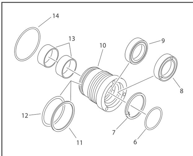
**Figure 5-37. Cylinder Head Disassembly**
