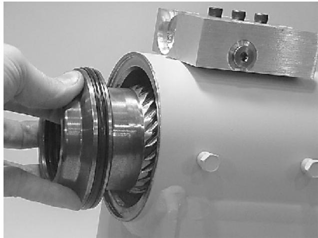
8. Looking from angle shown, rotate piston (3) until marks on piston and housing (1) made during disassembly line up as shown. Using a rubber mallet, tap piston into housing up to the point where gear teeth meet.
