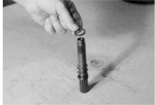
4. Stand input shaft (7A) on its splined end. Place one spacer (7D) on smooth end of input shaft (7A).
