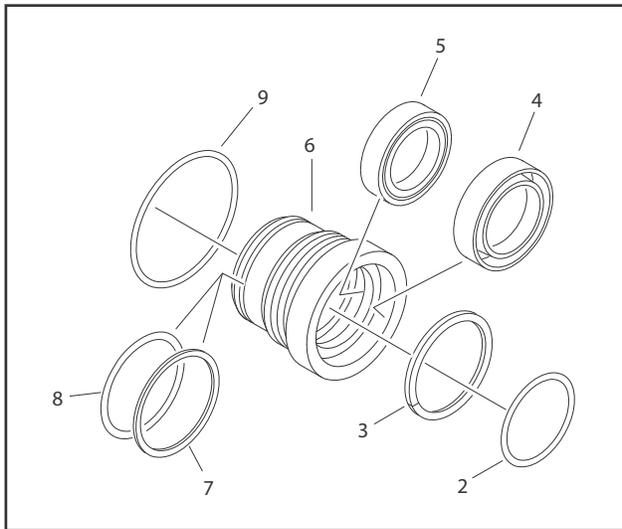
**Figure 5-67. Cylinder Head Assembly**
