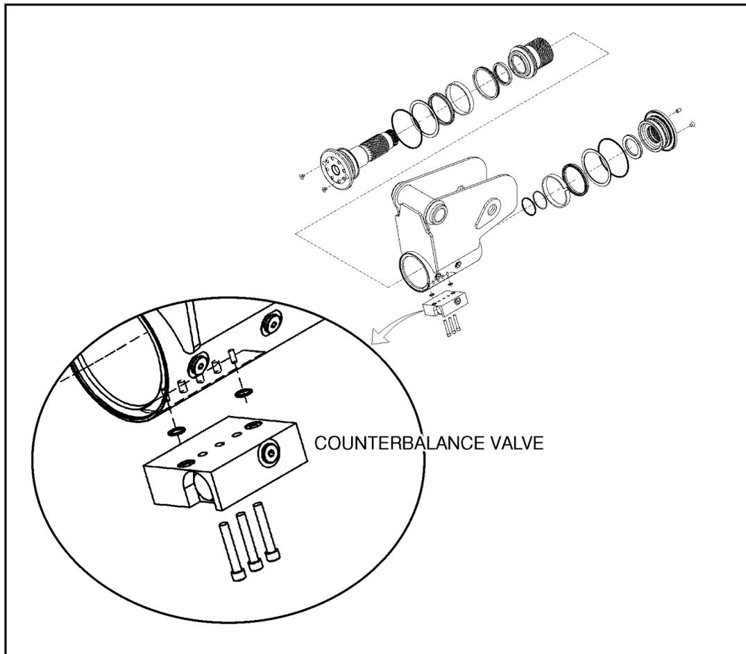
Figure 4-8. Rotator Counterbalance Valve
