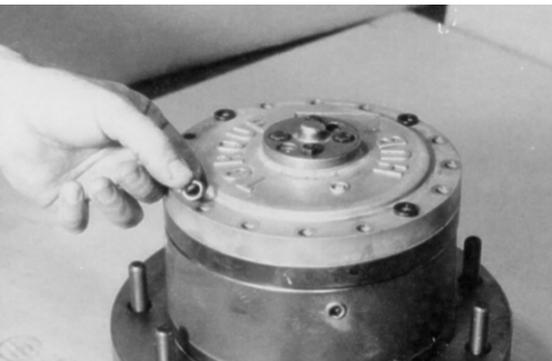
18. Place shoulder bolts (13) in four shoulder bolt holes in cover (6). Tighten by hand.
