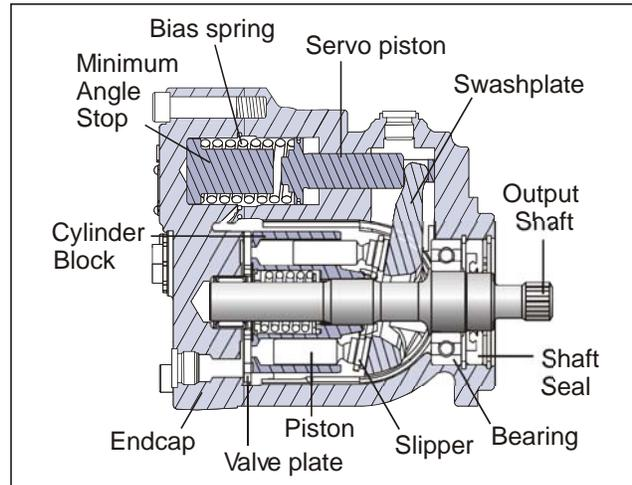
Figure 3-24. Drive Motor Cross Section
