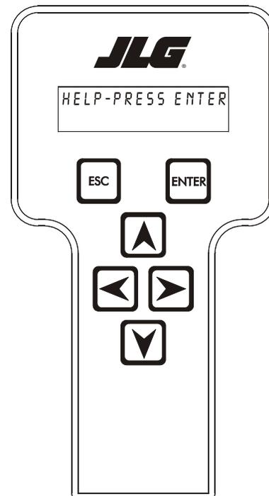
5. Use the arrow button to reach SYSTEM TEST. Hit Enter. The analyzer will prompt you asking if you want to activate the system test; hit Enter again to activate.
