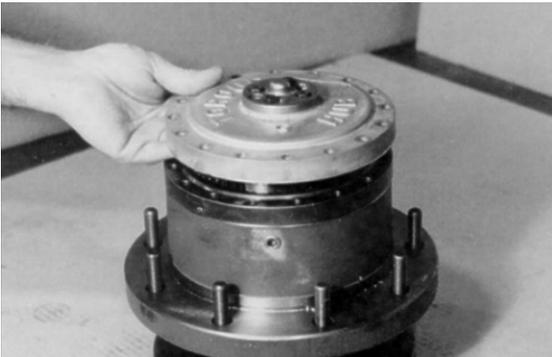
17. Place four flat washers (16) on top of bolt holes in cover sub-assembly.
