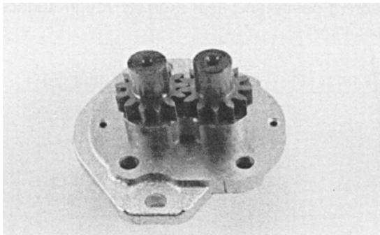
9. Install the idler gear shaft in the remaining position in the bearing block. Apply a light coat of clean oil to the face of the drive and idler gears.
