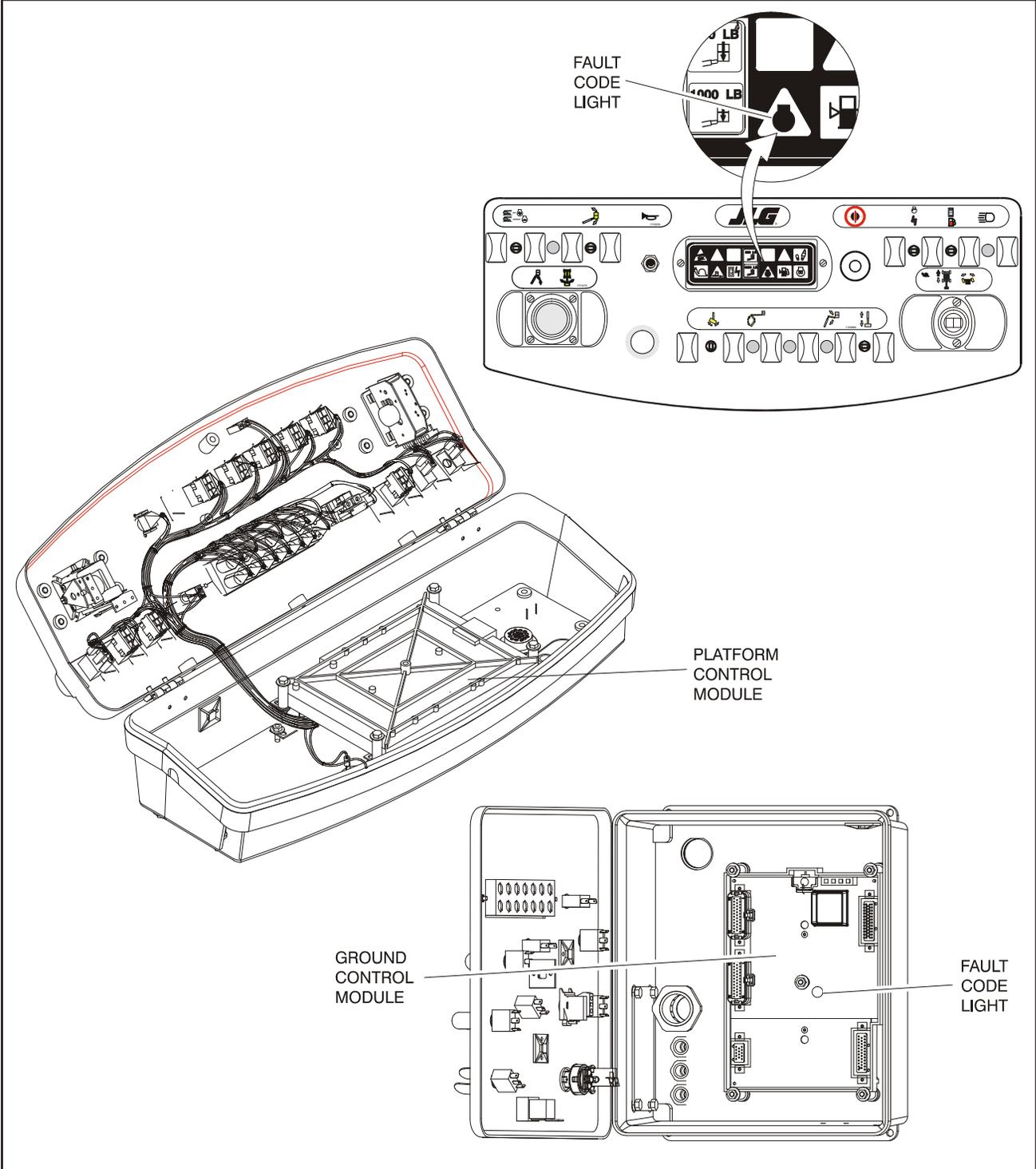
Figure 6-3. Control Module Location
