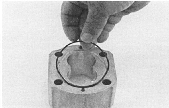
12. To install the O-rings in the gear housing, apply a light coating of petroleum jelly in the grooves on both sides of the gear housing. Also coat the new O-rings and install them in the grooves.
