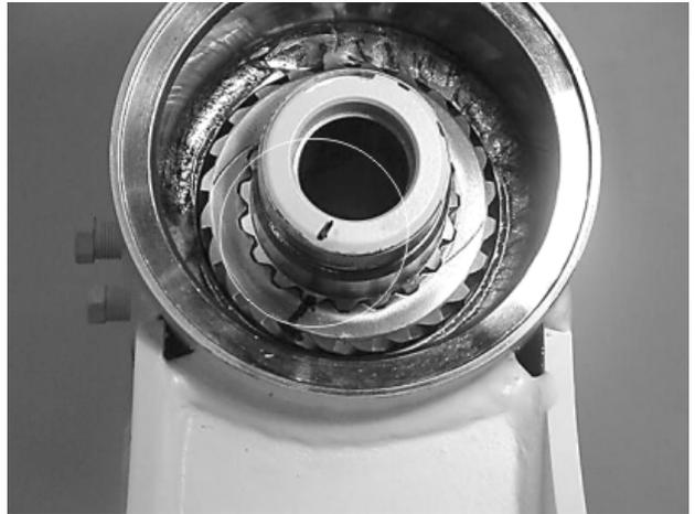
10. Remove shaft (2). It may be necessary to strike the threaded end of shaft with a rubber mallet.
