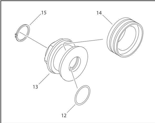
**Figure 5-45. Piston Disassembly**
