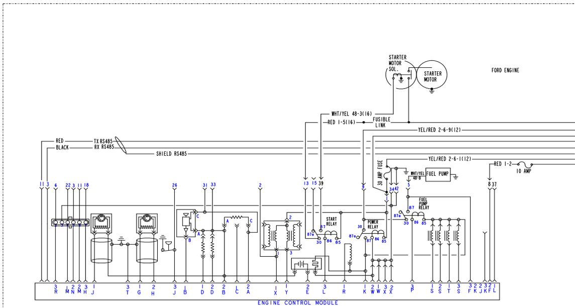
Figure 7-22. Electrical Schematic - Sheet 3 of 4
