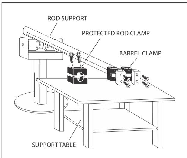
Figure 5-32. Cylinder Barrel Support
