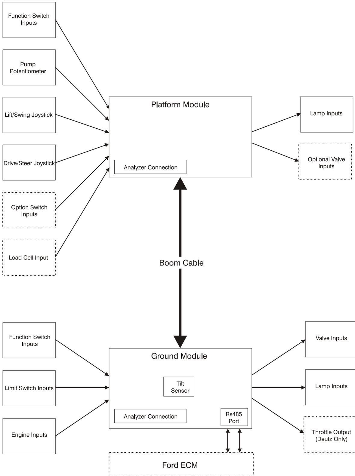
Figure 6-4. ADE Control System Block Diagram
