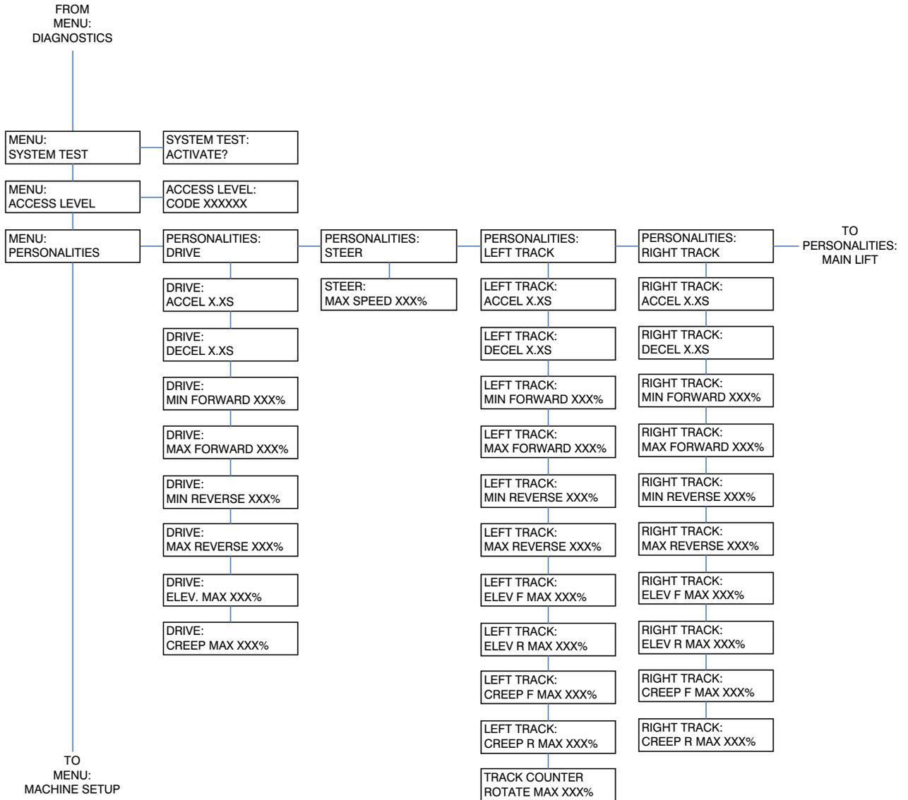
Figure 6-16. Analyzer Flow Chart, Version 6.X Software - Sheet 4 of 6
