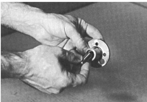
4. Set cover (6A) on table, exterior side up. Place cover cap (6B) on cover (6A), aligning pipe plug hole in cover cap over pipe plug hole in cover.
