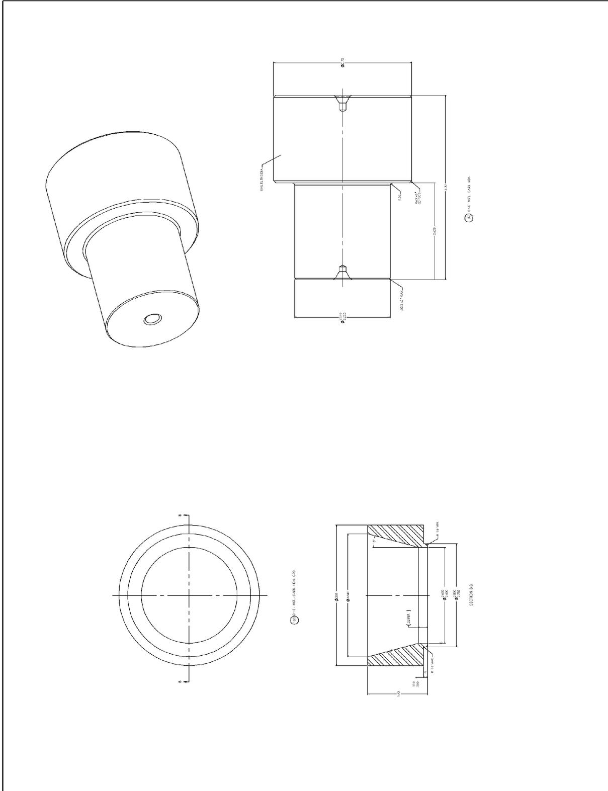
Figure 3-22. Assembly Tools - Brake Retaining Ring Installation
