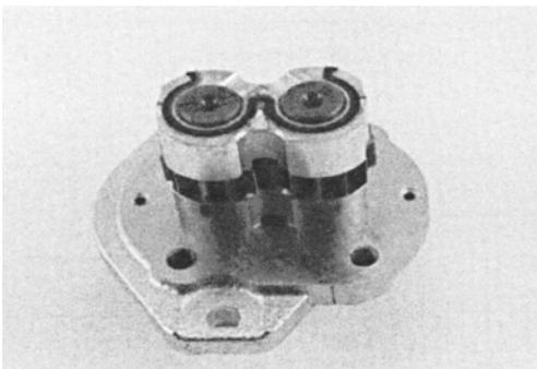
10. Pick up the rear bearing block, with seal side up and with open end of the E-seal facing the intake side of the pump, place over the drive and idler gear shafts.
