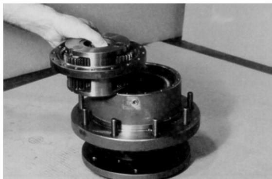
13. With internal splines facing up (counterbore end facing down), place input gear (8) into mesh with carrier sub-assembly (3).
