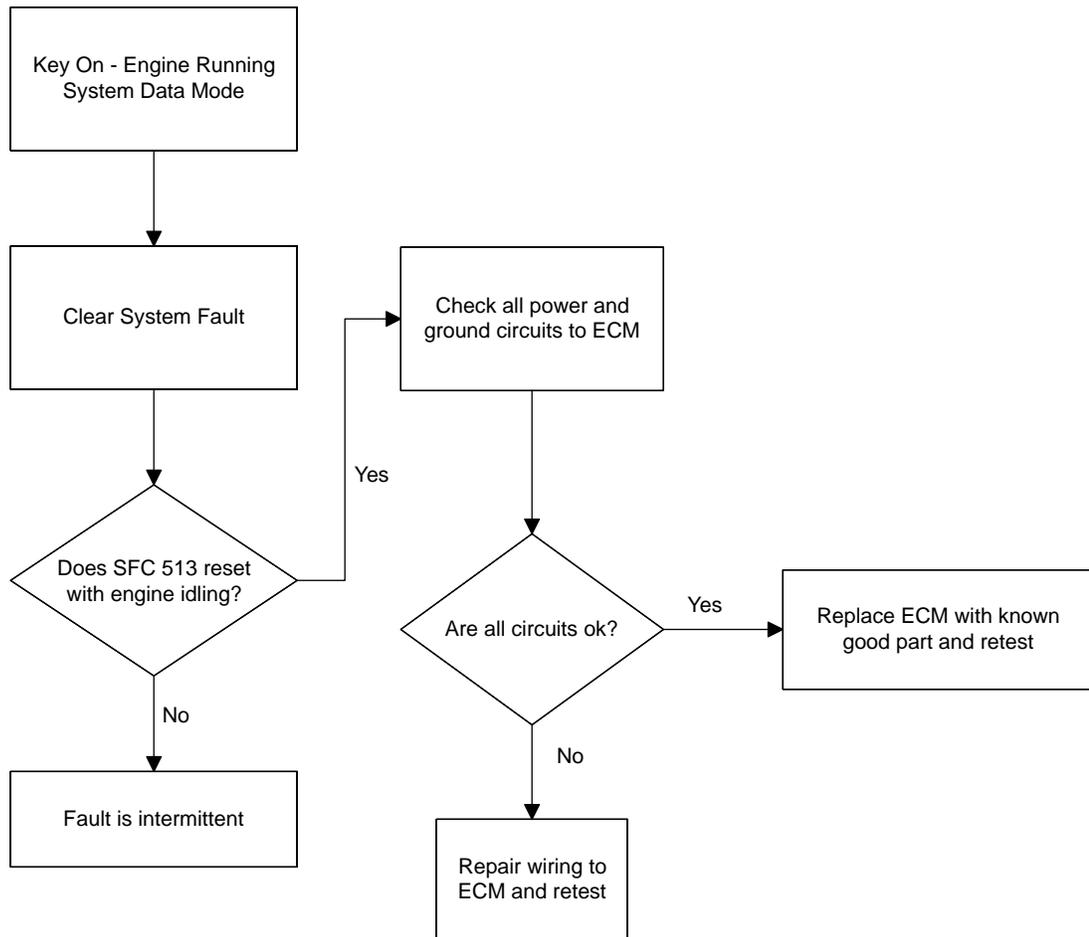
**DTC 1616- Microprocessor Failure - interrupt**
