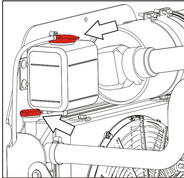
2. Fill radiator to the top. Allow enough time for coolant to properly settle in radiator and add coolant as necessary to top off.
