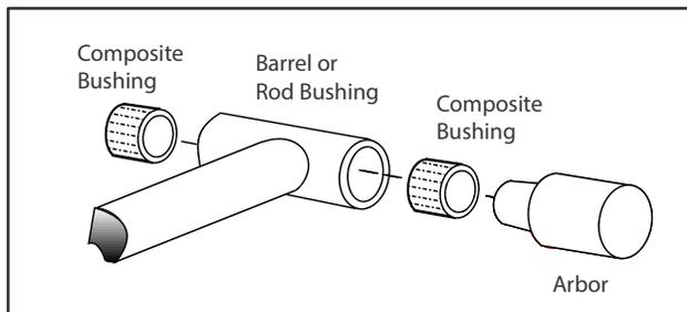
**Figure 5-77. Composite Bushing Installation**
