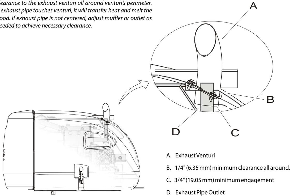
**Figure 3-78. Exhaust Venturi Adjustment**
