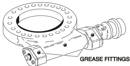
\*If necessary install grease fittings into worm gear housing and grease bearings.
