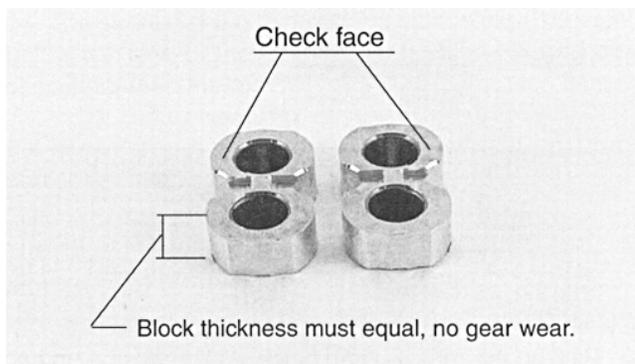
5. Inspect bearing blocks for excessive wear or scoring on the surfaces which are in contact with the gears. Also inspect the bearings for excessive wear or scoring.
