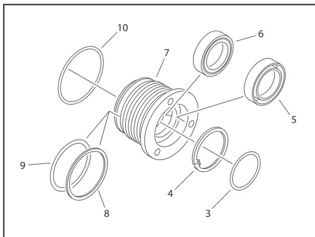
**Figure 5-27. Cylinder Head Disassembly**
