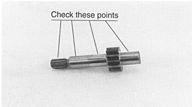
2. Check drive shaft spine for twisted or broken teeth, check keyed drive shaft for broken or chipped keyway. No marks or grooves on shaft in seal area, some discoloration of shaft is allowable.
