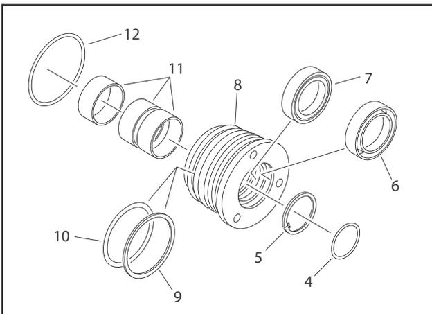
**Figure 5-17. Cylinder Head Disassembly**
