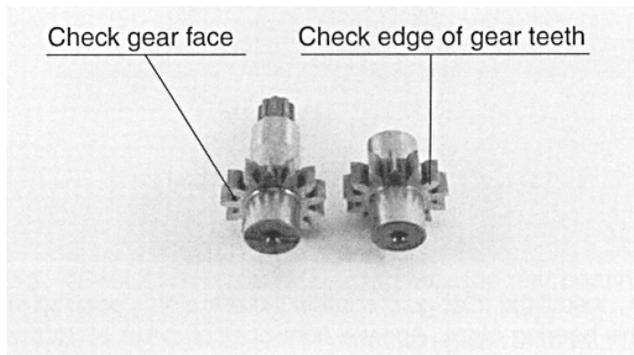
4. Inspect gear face for scoring or excessive wear. If the face edge of gear teeth are sharp, they will mill into the bearing blocks. If wear has occurred, the parts are unusable.
