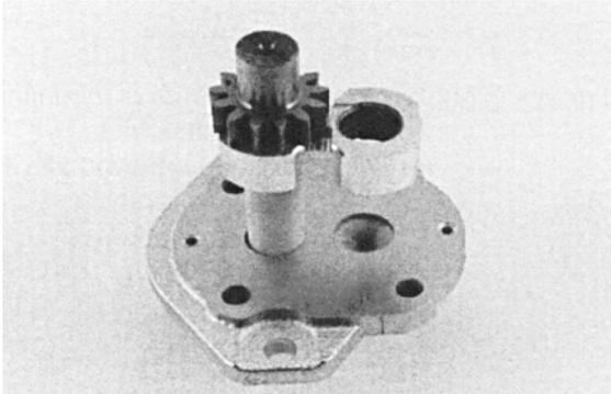
7. Insert the drive end of the drive shaft through the bearing block with the seal side down, and the open side of the E-seal pointing to the intake side of the pump.
