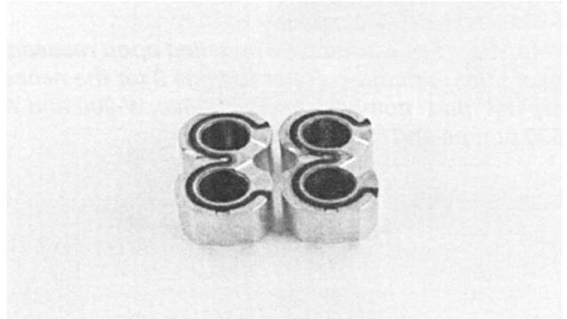
4. Place the E-seals, flat side outward, into the grooves in both bearing blocks. Follow by carefully placing the backup ring, flat side outward, in the groove made by the E-seal and the groove in the bearing block. (Note: in the W900 series pump, in the center of the backup ring and E-seal there is a notch make sure that these notches line up so the backup ring will set flush with the E-seal). The backup ring in the W1500 pump is symmetrical.
