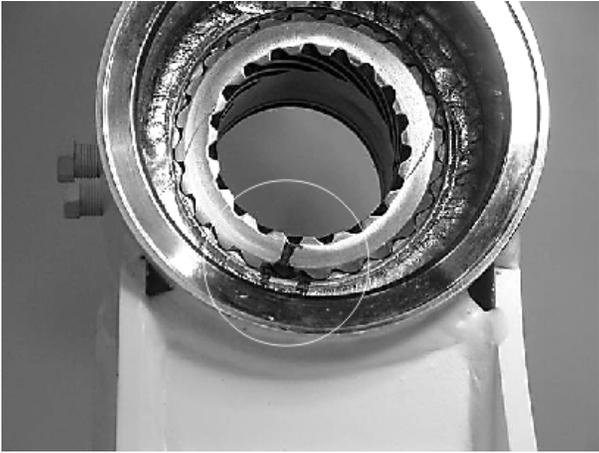
13. At the point when piston gear teeth come out of engagement with housing gear teeth, mark piston and housing with a marker as shown.
