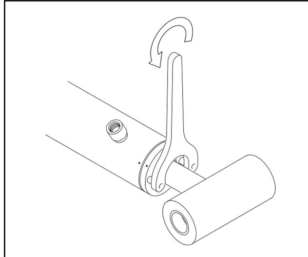
Figure 5-52. Cylinder Head Removal
