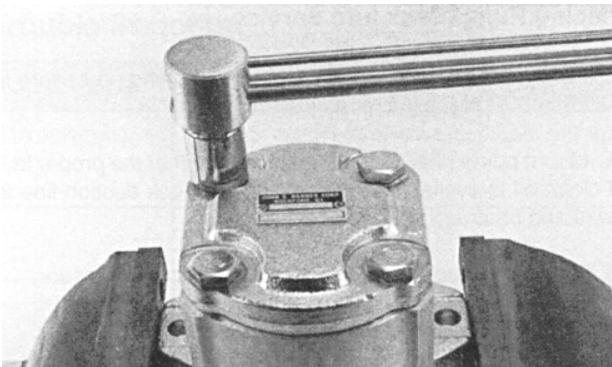
17. Place mounting flange of the pump back in the protected jawed vise and alternately torque the bolts to the torque specifications in the torque chart. All torque figures are for "dry torque" bolts.
