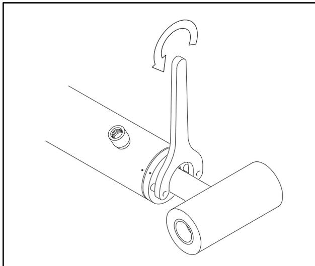
Figure 5-23. Cylinder Head Removal
