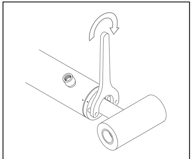
**Figure 5-60. Cylinder Head Installation**
