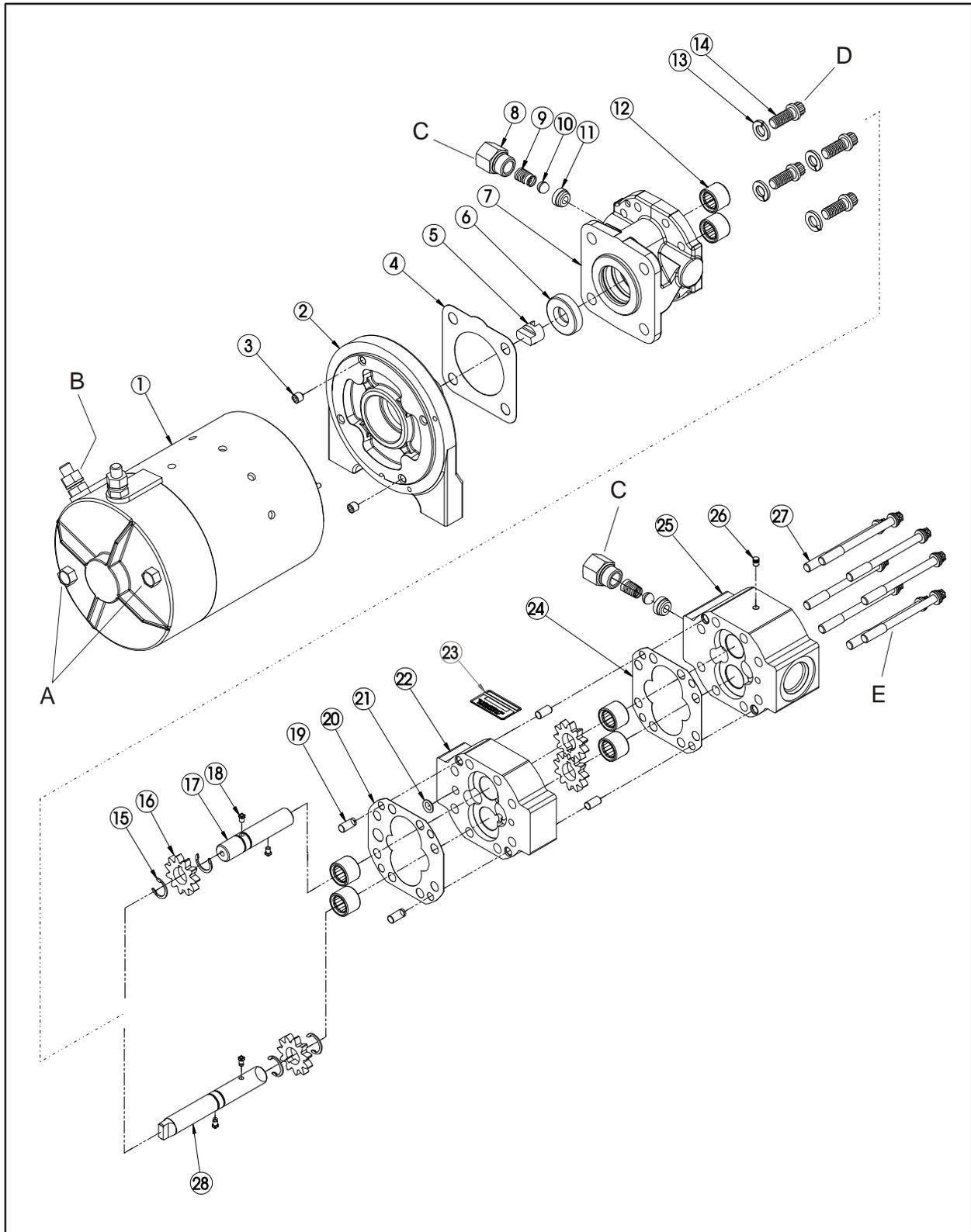
Figure 3-53. Auxiliary Pump - Sheet 1 of 2
