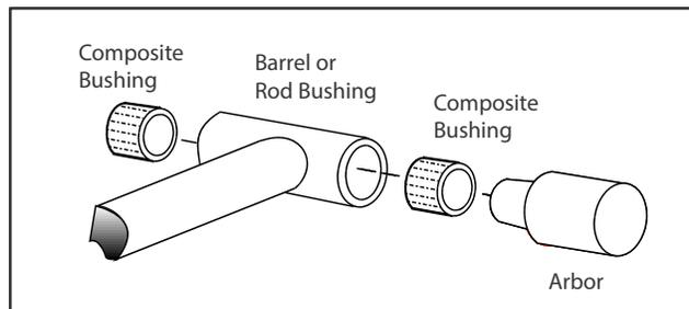
**Figure 5-18. Composite Bushing Installation**
