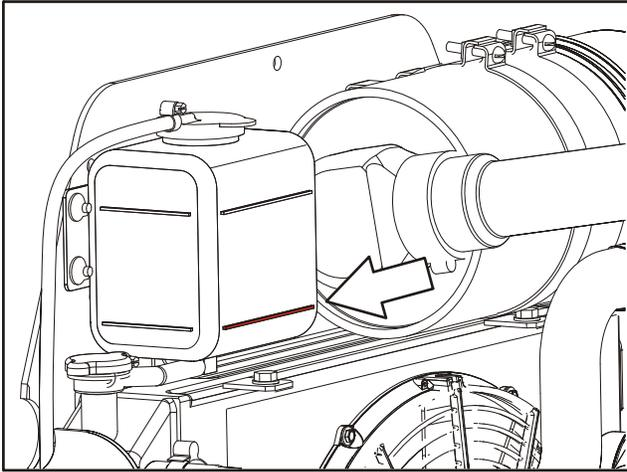
8. Make sure coolant reaches hot level line on coolant recovery reservoir. Add coolant as needed.
