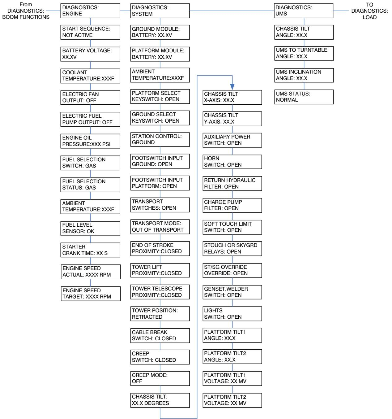
Figure 6-14. Analyzer Flow Chart, Version 6.X Software - Sheet 2 of 6
