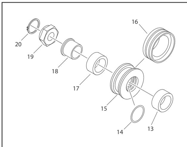
**Figure 5-55. Piston And Bushings Disassembly**
