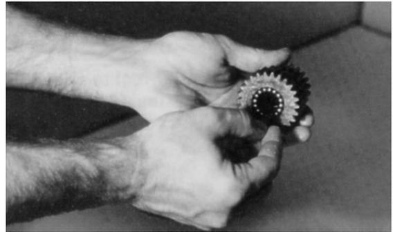
4. Set carrier housing (3A) on table, sideways. Insert a planet shaft (3E), roll pin hole last, in one of planet shaft holes from roll-pin-holed side of carrier housing (3A).
