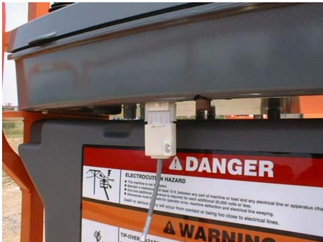
3. Pull out Emergency Stop switch and Start engine.
