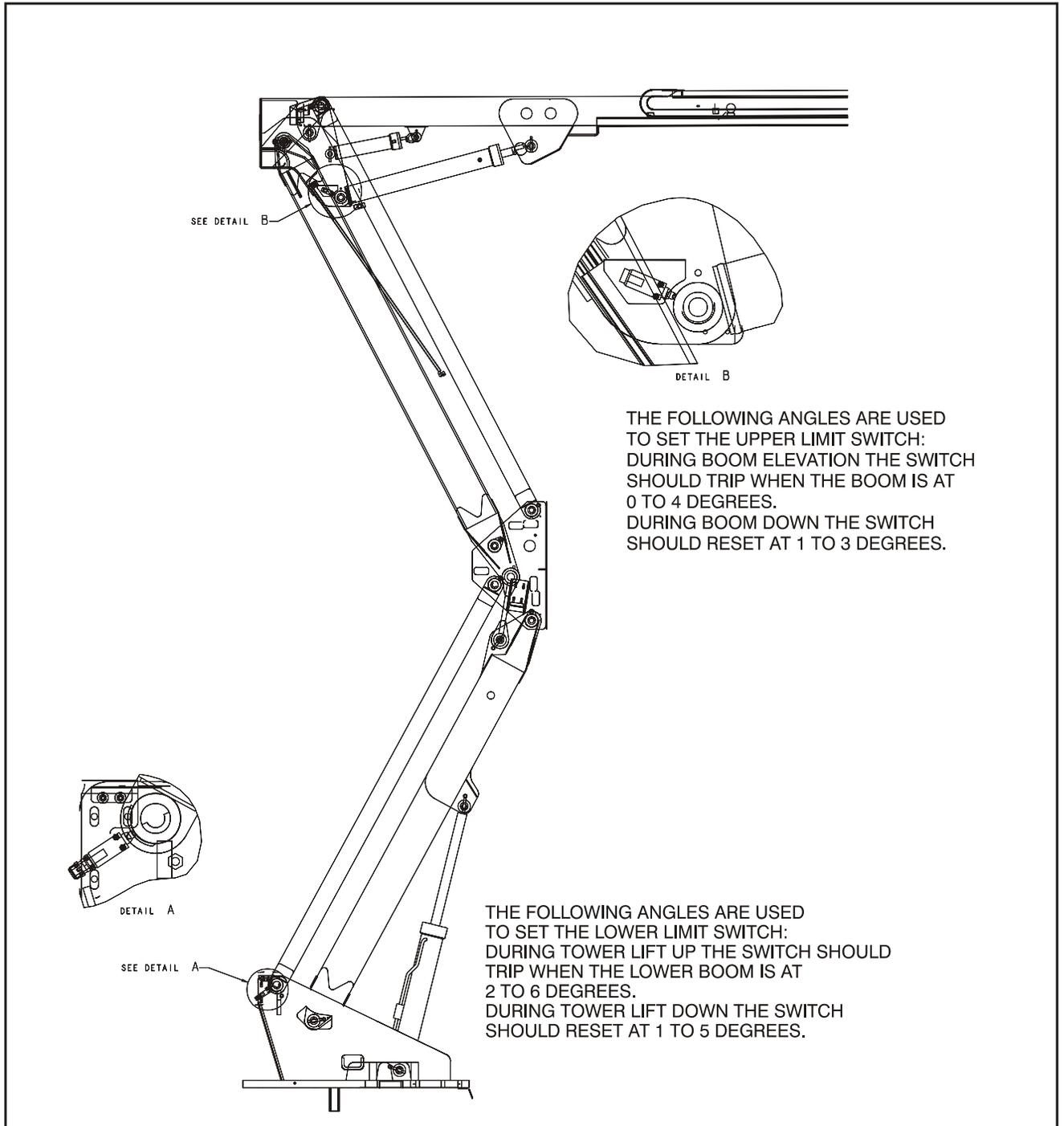
Figure 4-2. Boom Limit Switches
