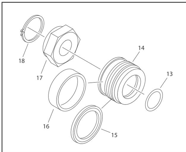
**Figure 5-75. Piston Disassembly**
