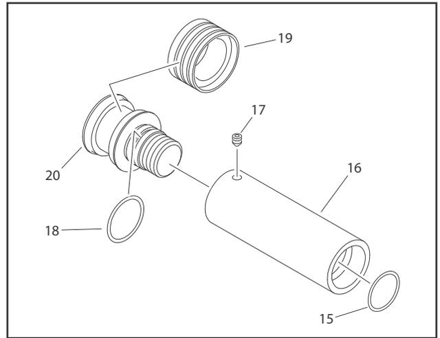
**Figure 5-39. Piston And Spacer Assembly**
