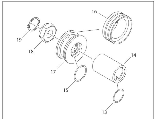
**Figure 5-10. Piston And Spacer Assembly**
