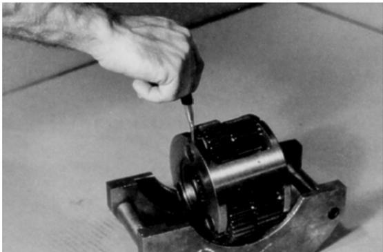
9. Drive roll pin (3G) down in aligned roll pin holes in carrier housing (3A) and planet shaft (3E).
