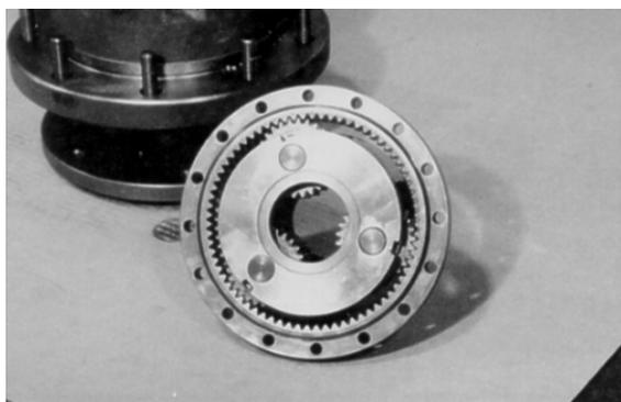
12. Place carrier sub assembly (3) and ring gear (4) together into mesh with internal gear (2). Align "X" marked shoulder bolt hole in ring gear (4) over one of the shoulder bolt holes in the hub. Mark location of shoulder bolt holes on outside of ring gear and hub.
