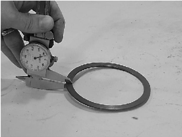
3. Inspect wear guide condition and measure thickness (not less than 0.123" or 3.12 mm).
