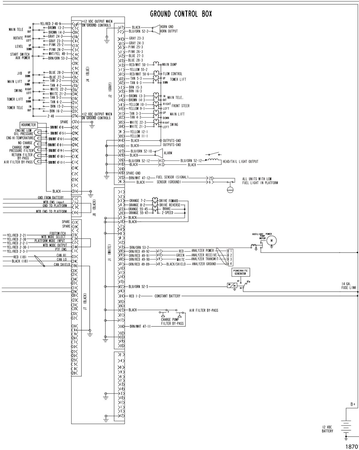
Figure 7-21. Electrical Schematic - Sheet 2 of 4
