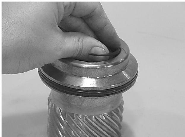
7. Insert piston (3) in housing (1) as shown, until outer piston seal (202) is touching inside housing bore.
