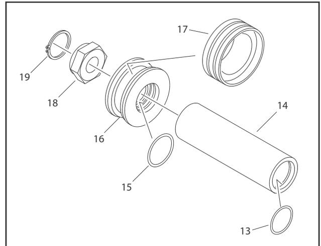
**Figure 5-20. Piston And Spacer Assembly**
