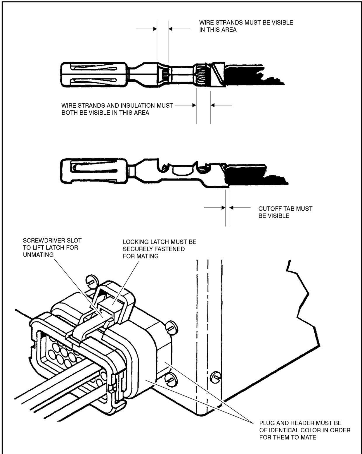
Figure 7-11. Connector Installation
