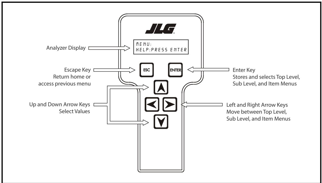
Figure 6-1. Hand-Held Analyzer (WANALYZER Controls and Display Similar)
