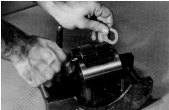
8. Use an alignment punch or similar tool to align roll pin holes in carrier housing (3A) and planet shaft (3E).
