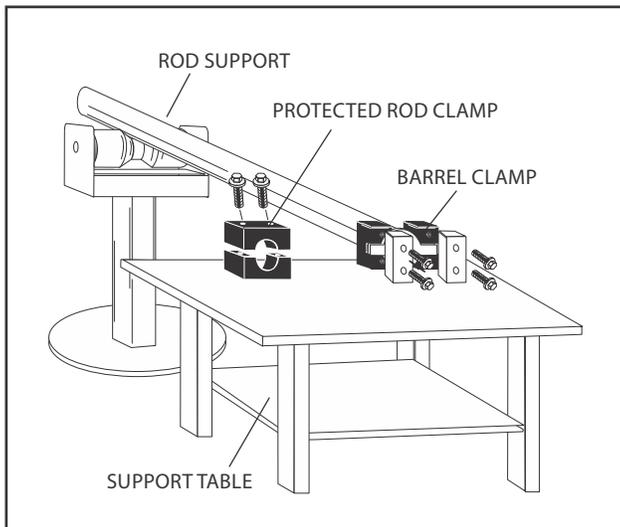
Figure 5-51. Cylinder Barrel Support
