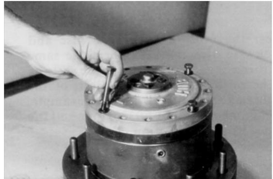
19. Place remaining 12 flat washers (16) on remaining bolt holes in cover (6).
