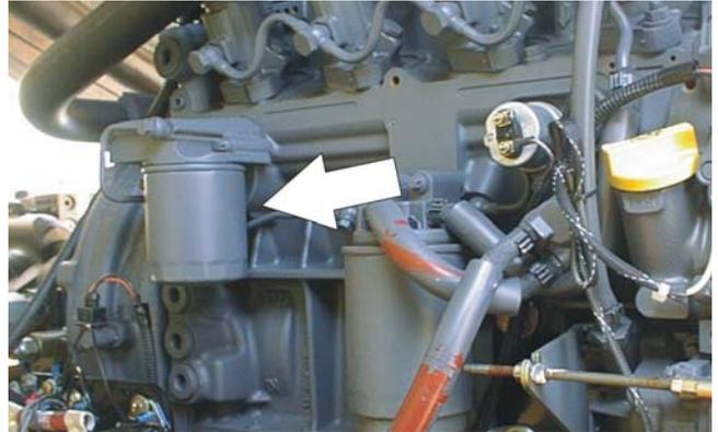
Lube Point(s) - Fill Cap/Spin-on Element
