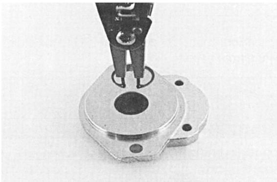
2. Install retaining ring in groove in seal bore of mounting flange.
