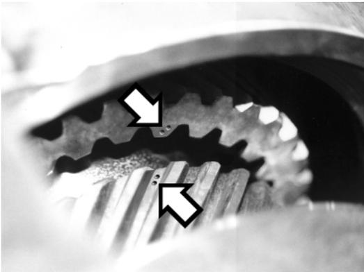
9. Before removing shaft, (2), use a felt marker to clearly indicate timing marks between shaft and piston. This will greatly simplify timing during assembly.
