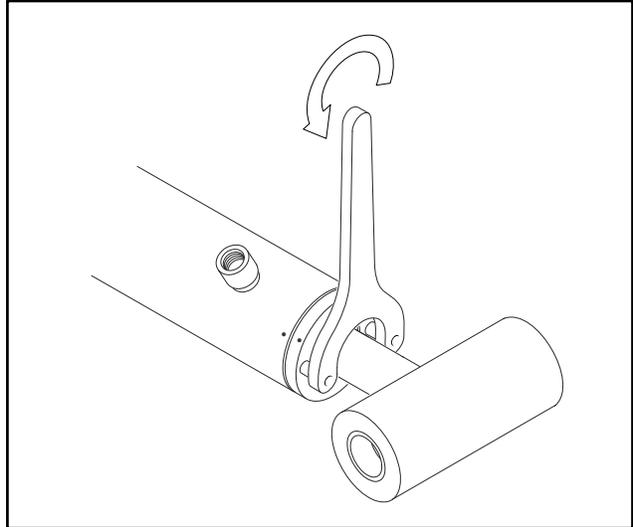
Figure 5-33. Cylinder Head Removal
