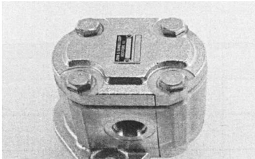
16. Install the four spacers, if applicable, and hex head bolts through the bolt holes in the end cover, hand tighten.
