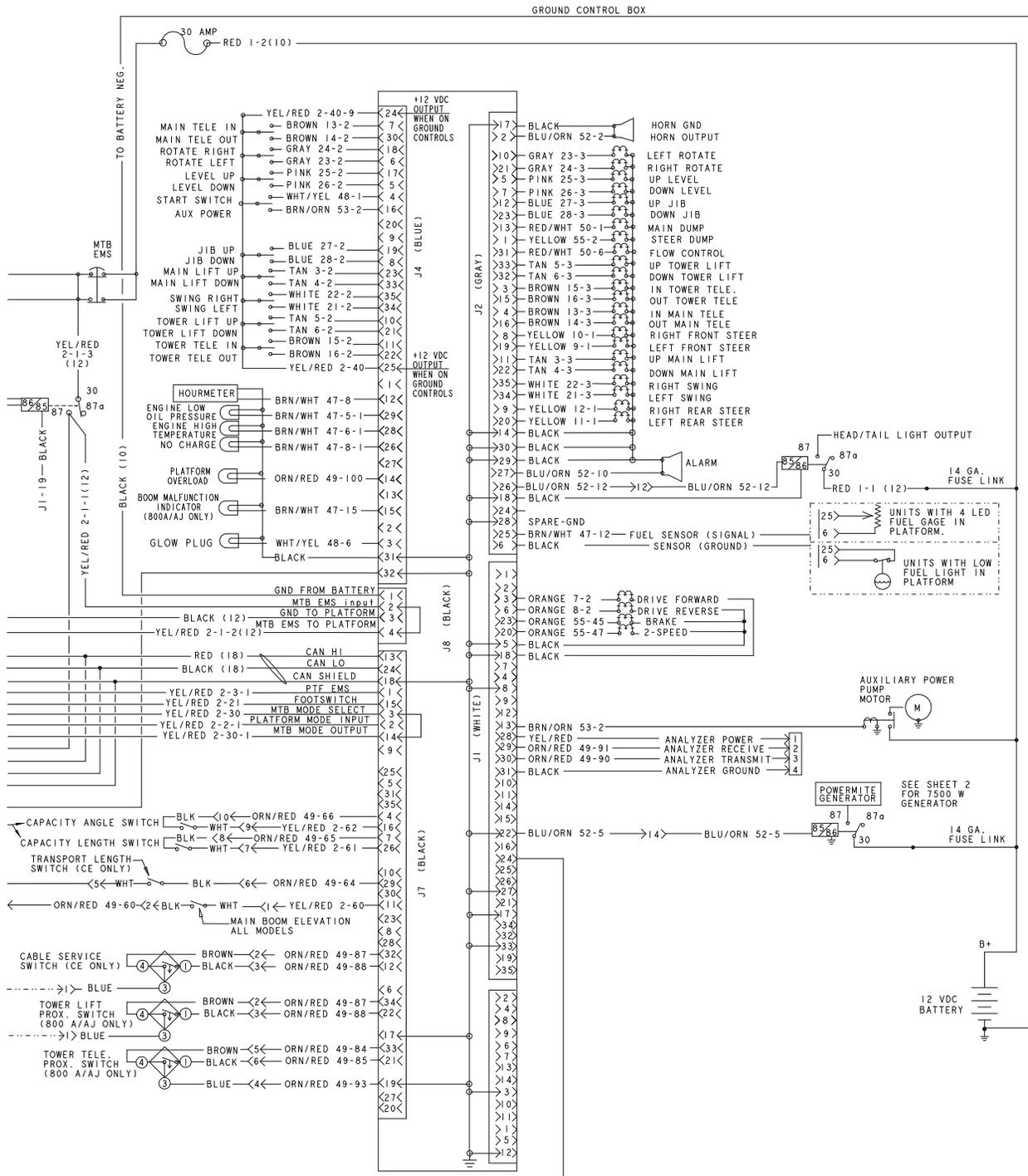
Figure 7-25. Electrical Schematic - Deutz EMR2 & GM Engine - Sheet 2 of 6
