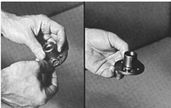
3. Insert disconnect rod (6E) in cover cap (6B).
