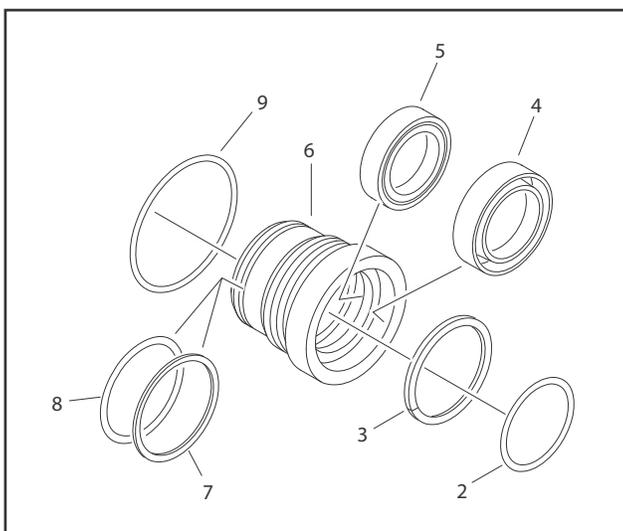
**Figure 5-66. Cylinder Head Disassembly**
