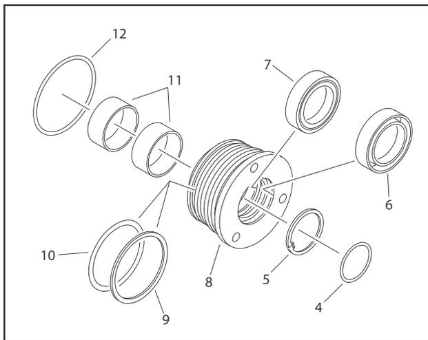
**Figure 5-9. Cylinder Head Assembly**
