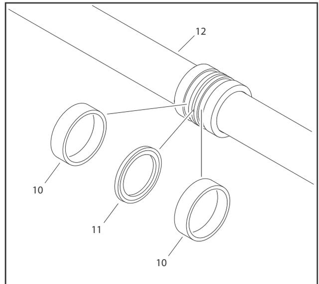
**Figure 5-68. Piston Seal and Wear Ring**
