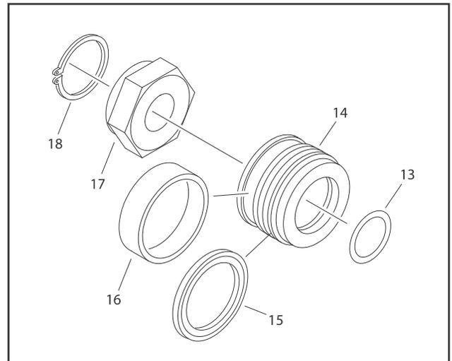
**Figure 5-79. Piston And Bushings Assembly**
