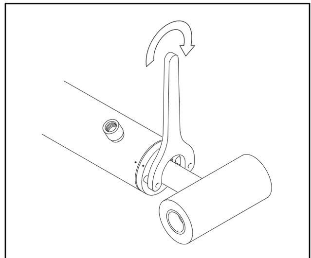
**Figure 5-21. Cylinder Head Installation**
