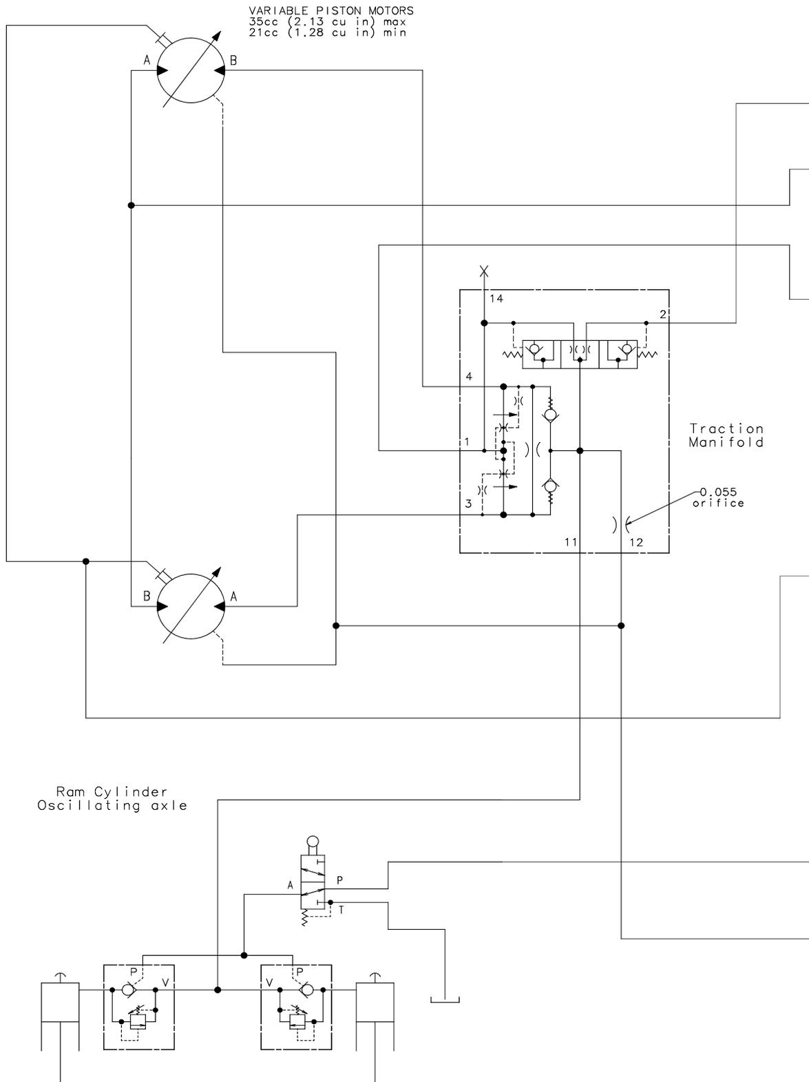
**Figure 5-92. Hydraulic Schematic - Sheet 3 of 6**
