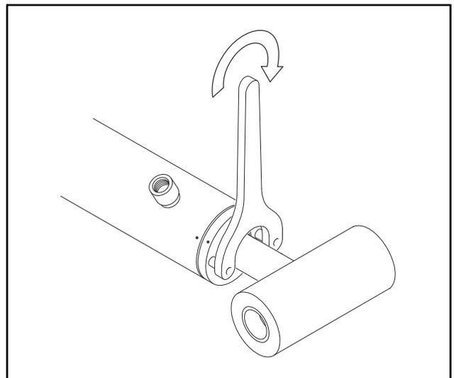
**Figure 5-40. Cylinder Head Installation**
