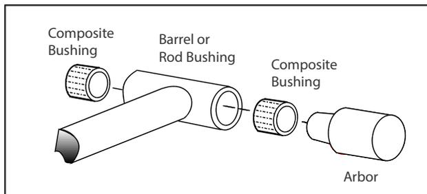
**Figure 5-57. Composite Bushing Installation**
