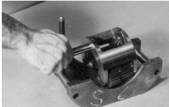
5. Place one thrust washer (3B) onto the end of planet shaft (3E) inside carrier. Fit tang of thrust washer into the slot on the inside edge of the planet shaft hole.
