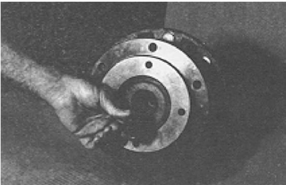
23. Roll test unit in clockwise and counterclockwise directions. Perform same number of turns in each direction as the ratio of the unit. The ratio is last two digits of model number on the unit's ID tag.
