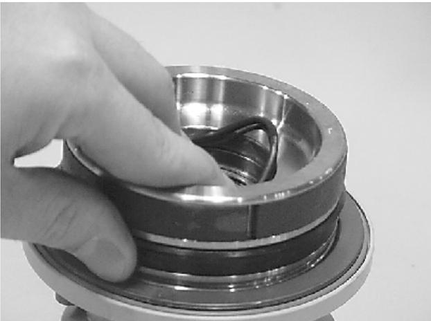
16. Thread end cap (4) on shaft (2) end. Make sure wear guide stays in place on end cap as it is threaded into housing (1).
