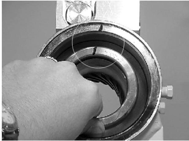
12. To remove piston (3) use a rubber mallet and a plastic mandrel so piston is not damaged.
