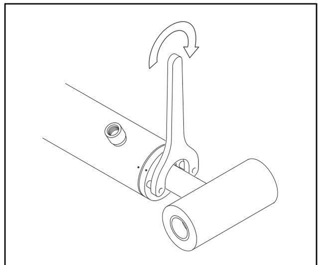
**Figure 5-11. Cylinder Head Installation**
