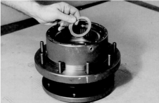
6. Place spacer (7D) on smooth end of input shaft (7A).
