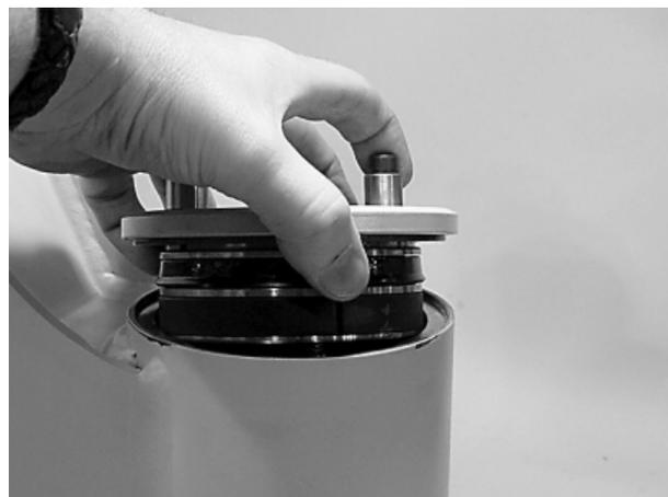
7. Remove stop tube if included. Stop tube is an available option to limit rotation of the actuator.
