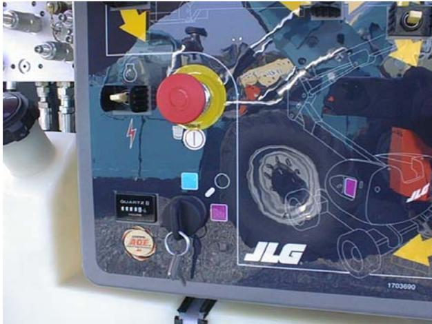
2. Plug analyzer in connector at base of platform control box.
