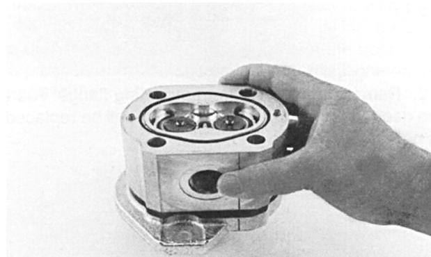
9. Carefully remove gear housing and place on work bench. Make sure the rear bearing block remains on the drive and idler shafts.
