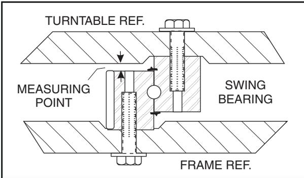
Figure 3-51. Swing Bearing Tolerance Measuring Point
