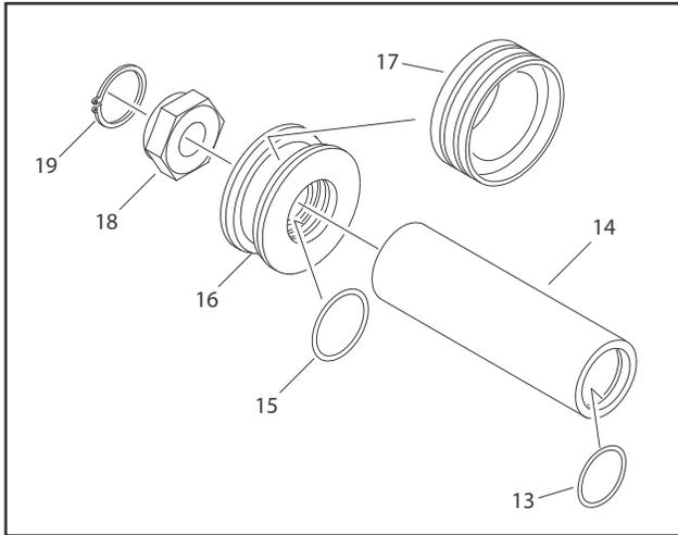
**Figure 5-16. Piston And Spacer Disassembly**
