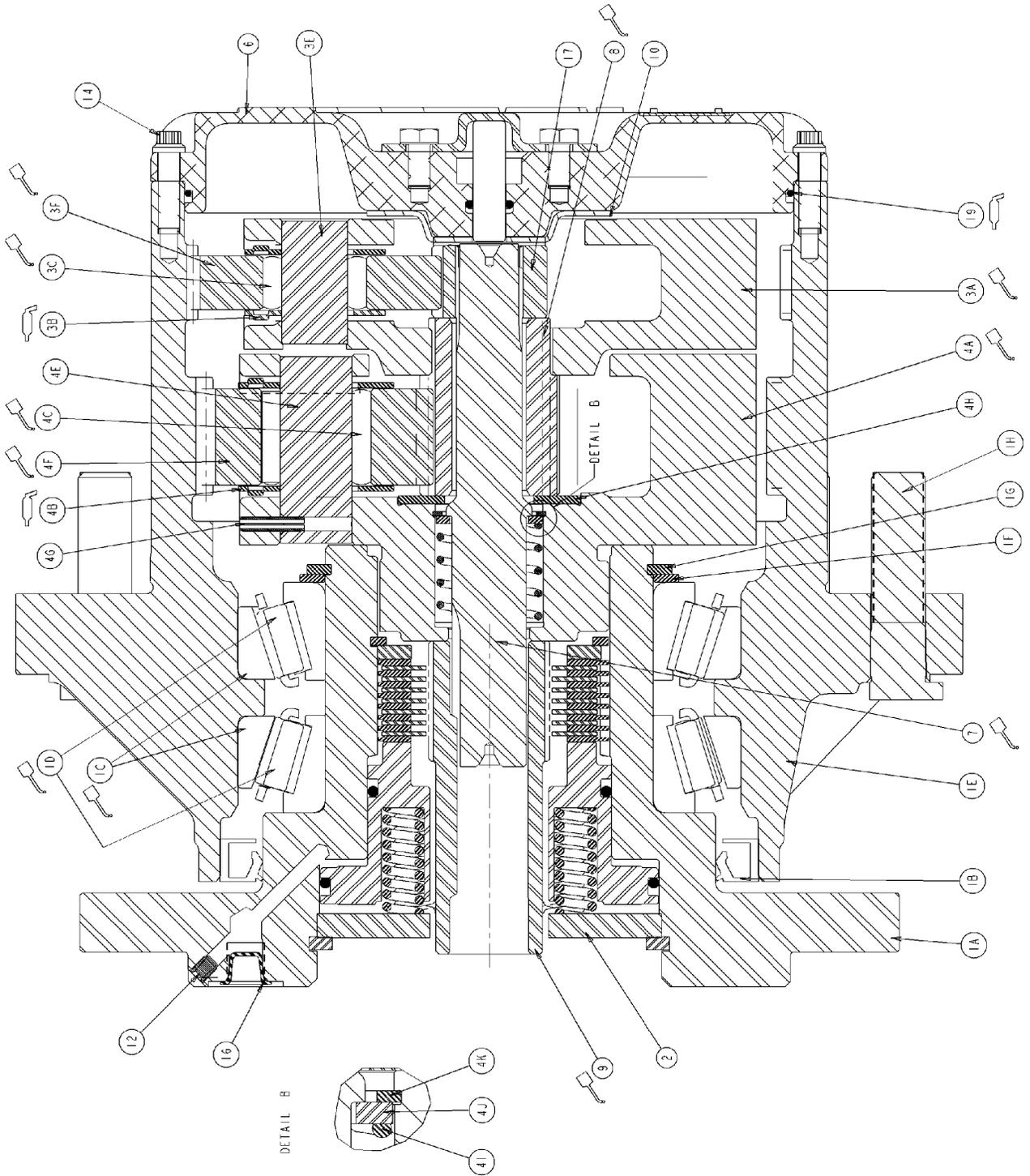
Figure 3-15. Assembly Drawing - With Integral Input Brake - Sheet 1 of 2
