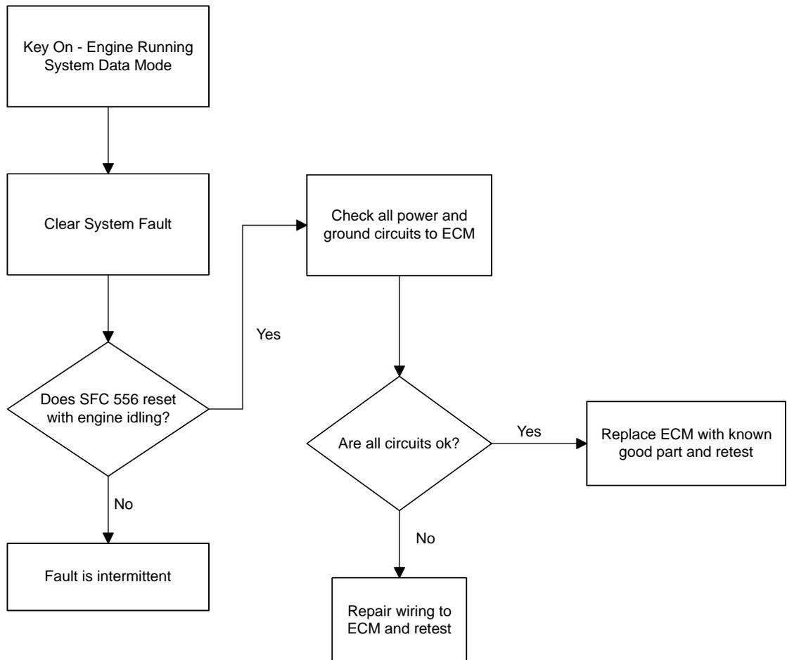
**DTC 1615- Microprocessor Failure - A/D**
