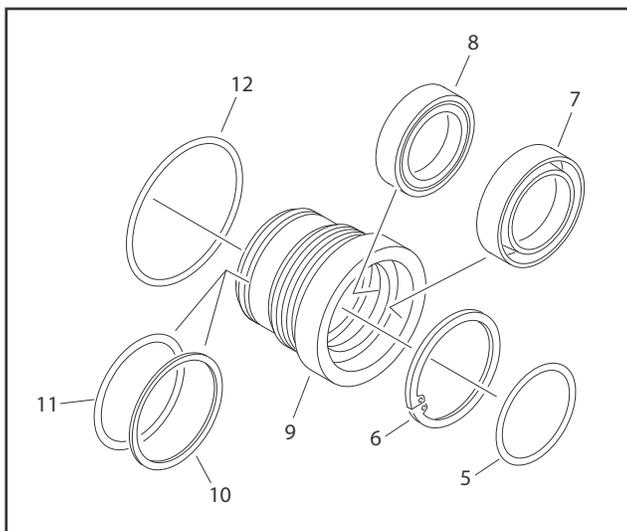
**Figure 5-76. Cylinder Head Disassembly**
