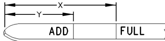
**NOTE:** Operating your engine when oil level is above "FULL" mark could cause your crankshaft to dip into the oil. Air bubbles created from crankshaft dipping into the oil reduces the oil's lubricating characteristics and could result in loss of power.
