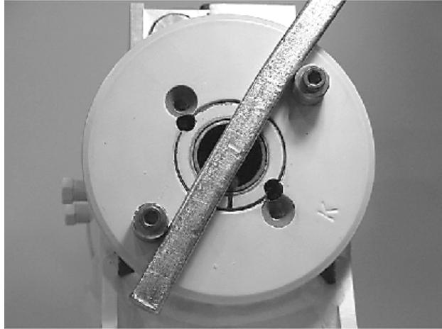
18. Place lock pins (109) provided in Helac seal kit in holes with dimple side up. Using a punch, tap lock pins to bottom of hole.
