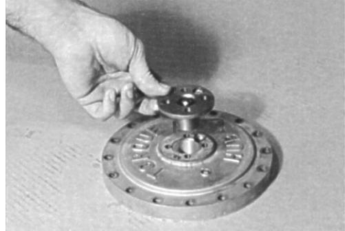
5. Place two cover cap bolts (6C) in any two bolt holes that are 180° apart on cover cap (6B) and tighten bolts.
