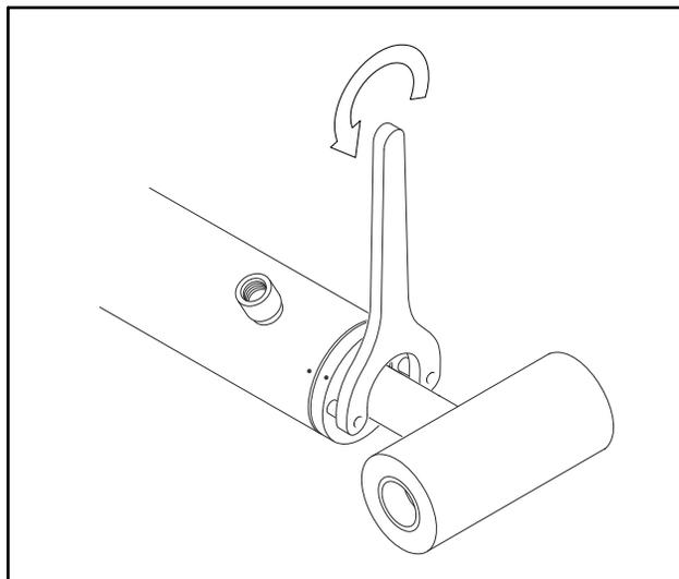
Figure 5-13. Cylinder Head Removal
