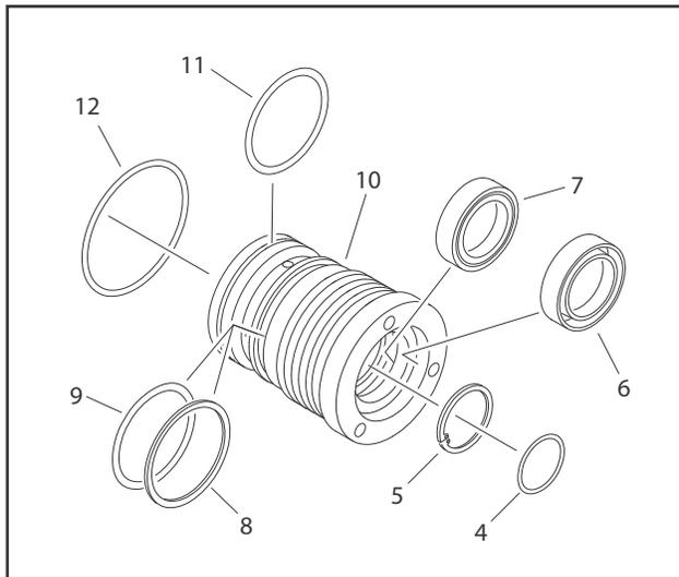
**Figure 5-58. Cylinder Head Assembly**
