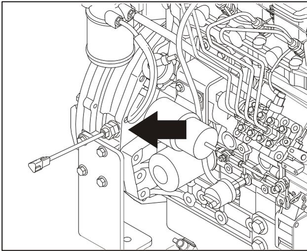
3. Back off the sensor 1/4 to 3/4 turn and ensure the sensor flats are vertical and tighten the nut.
