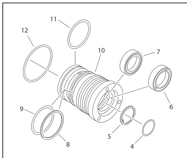
**Figure 5-56. Cylinder Head Disassembly**
