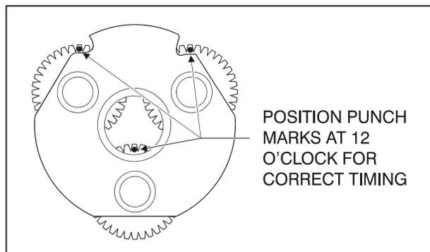
**Figure 3-23. Cluster Gear Punch Marks**
