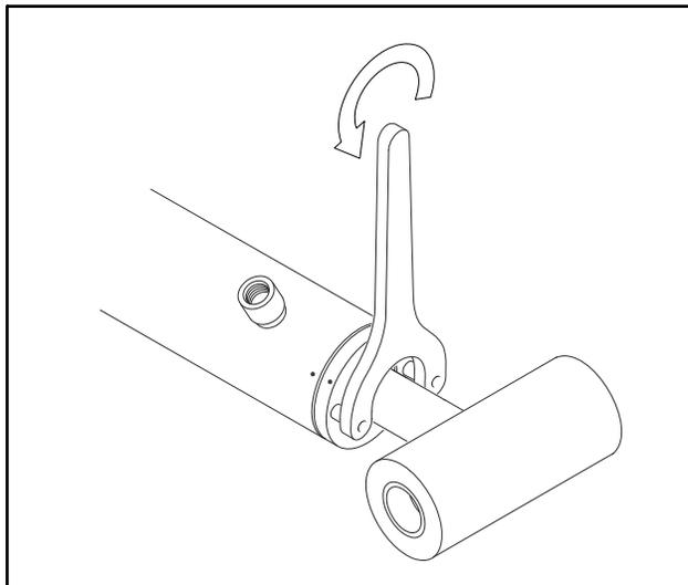
Figure 5-3. Cylinder Head Removal
