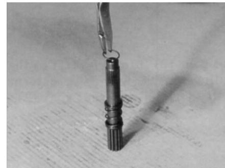
8. With large splined end down, place input shaft sub-assembly (7) in spindle (1A).
