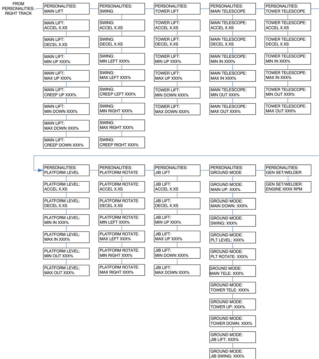
Figure 6-17. Analyzer Flow Chart, Version 6.X Software - Sheet 5of 6
