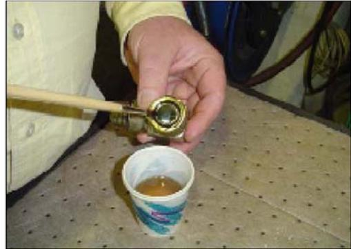
3. Turn fitting over and repeat previous step to O-ring on other side of fitting. Make sure entire O-ring is coated with hydraulic oil.
