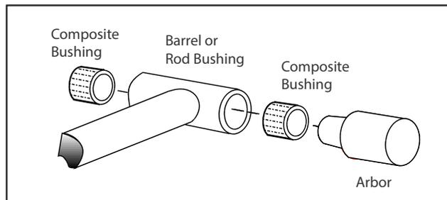
**Figure 5-8. Composite Bushing Installation**
