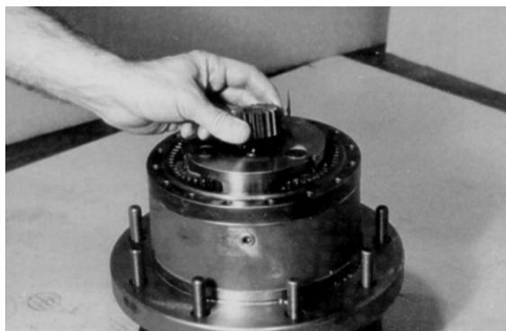
14. Oil all exposed surfaces inside hub (1G). Place thrust washer (11) in counterbore in top of carrier.
