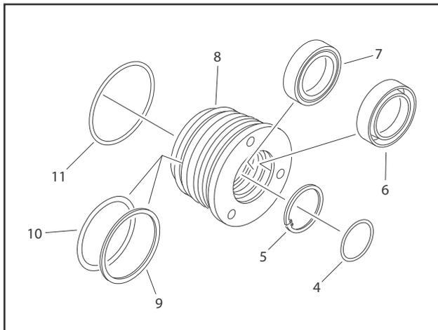
**Figure 5-48. Cylinder Head Assembly**
