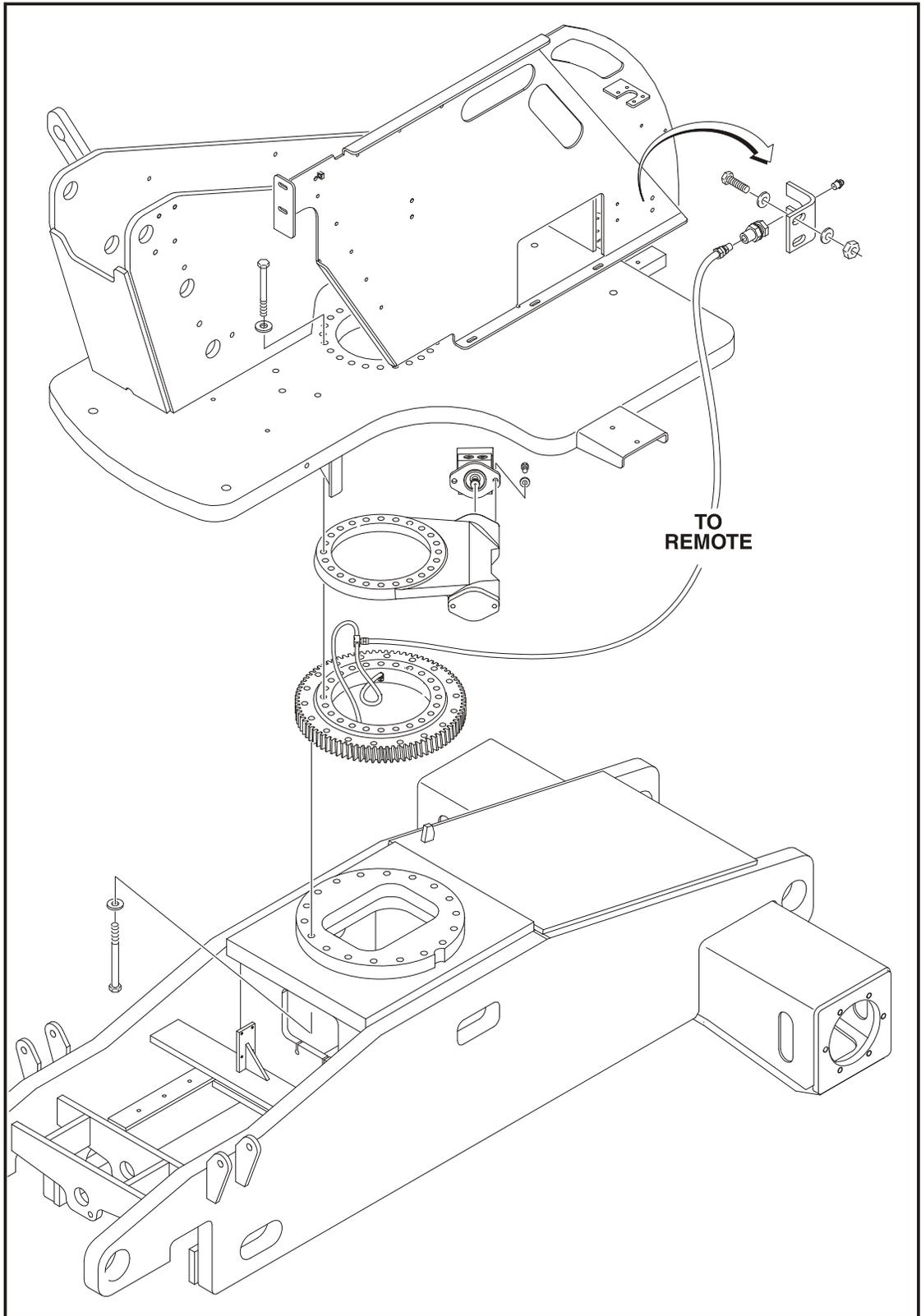
Figure 3-48. Swing Bearing Installation
