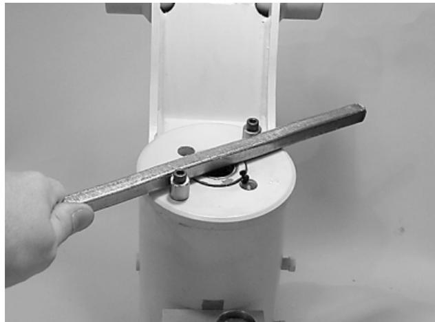
6. Remove end cap (4) and set aside for later inspection.
