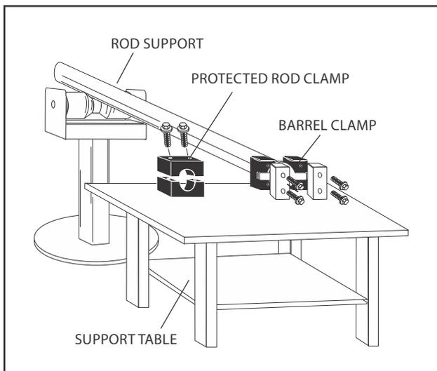
Figure 5-22. Cylinder Barrel Support
