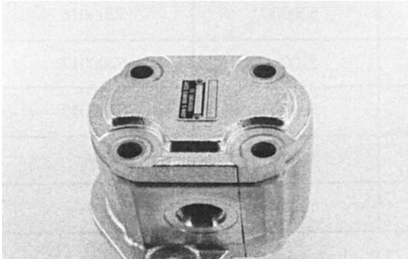
15. Install the two remaining dowel pins in the rear of the gear housing, if applicable, and place the end cover over the back of the pump.
