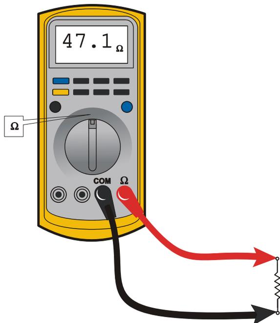
**Figure 7-2. Resistance Measurement**
