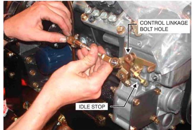
3. Once the adjustments have been made to align the spherical rod end bearing with the control linkage bolt hole, lengthen the actuator linkage by continuing to turn the spherical rod end and threaded rod 2-2 ½ turns (1-1 ¼ turns of spherical rod end and 1-1 ¼ turns of threaded rod.) This will provide 1/8" (3 mm) preload.
