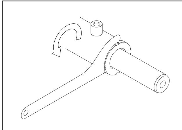
Figure 5-72. Cylinder Head Removal
