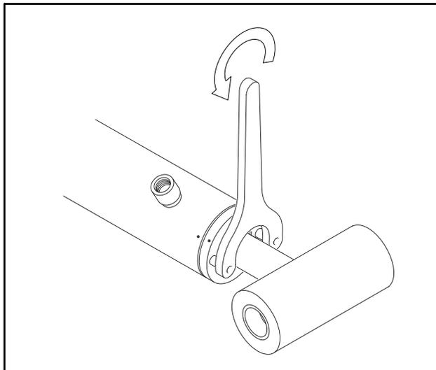
Figure 5-42. Cylinder Head Removal
