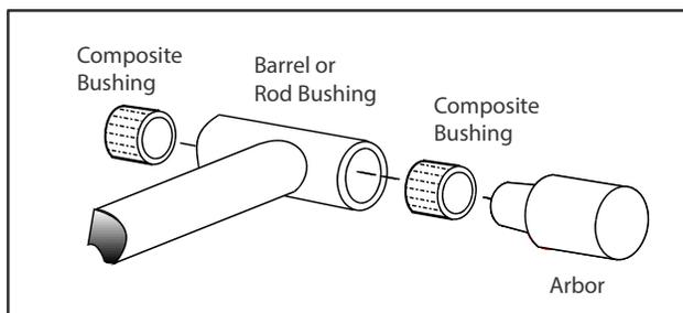
**Figure 5-28. Composite Bushing Installation**
