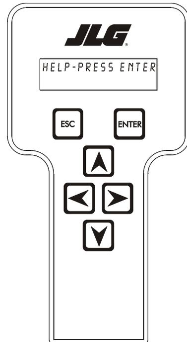
5. Use arrow button to reach SYSTEM TEST. Hit Enter. The analyzer will prompt if you want to activate system test; hit Enter again to activate.
