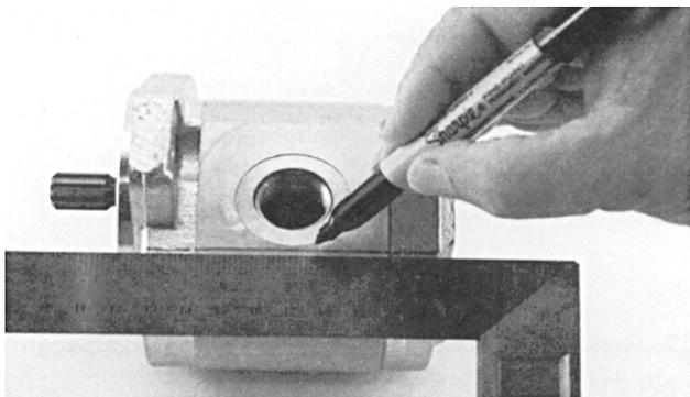
3. Use a permanent marker pen to mark a line across the mounting flange, gear housing and end cover. This will assure proper reassembly and rotation of pump.
