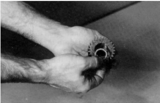
3. Line remaining half of cluster gear (3F) with 16 needle rollers.
