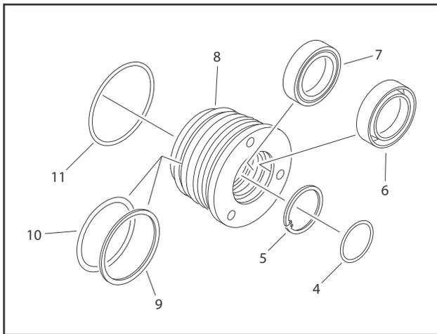
**Figure 5-46. Cylinder Head Disassembly**
