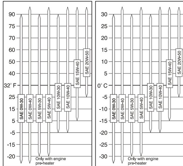
**Figure 3-55. Engine Oil Viscosity**
