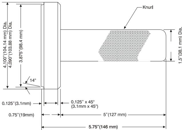
3. T-140433 ASSEMBLY PRESSING TOOL for CUP (1E)
