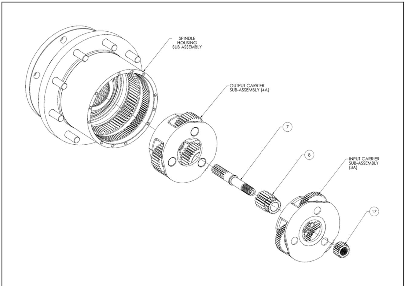
7. Input Shaft      8. Output Sun Gear      17. Input Sun Gear
