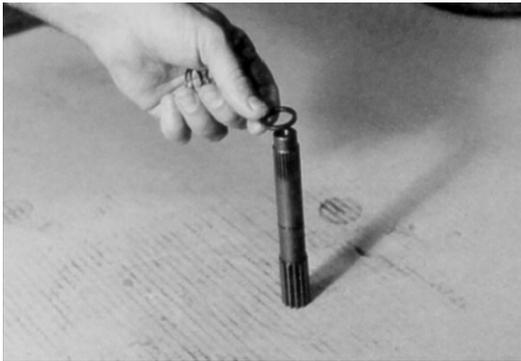
5. Place one spring (7C) on smooth end of input shaft (7A).
