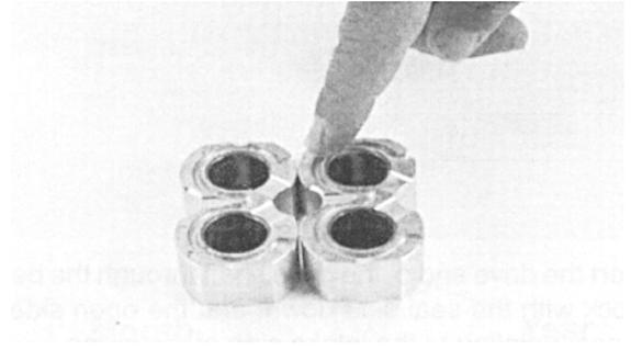
3. Place front and back bearing blocks on a clean surface with the E-seal grooves facing up. Apply a light coating of petroleum jelly in the grooves. Also coat the E-seal and backup with the petroleum jelly, this will help keep the seals in place during reassembly.
