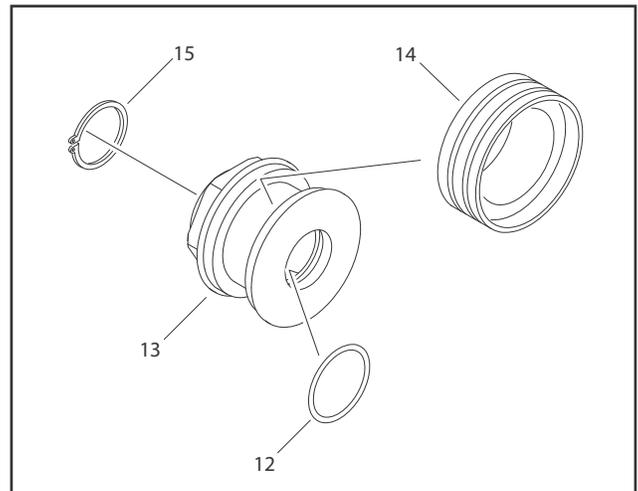
**Figure 5-49. Piston And Spacer Assembly**
