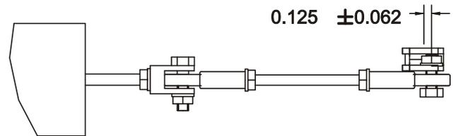
Use a measuring device to ensure the preload is approximately 1/8" (3 mm), then secure the actuator linkage to the control linkage with original bolt and nut. Make sure the spherical ball is seated in the control linkage bolt hole. Tighten two nuts on the threaded rod of the actuator linkage and using two wrenches to prevent binding of clevis heads.
