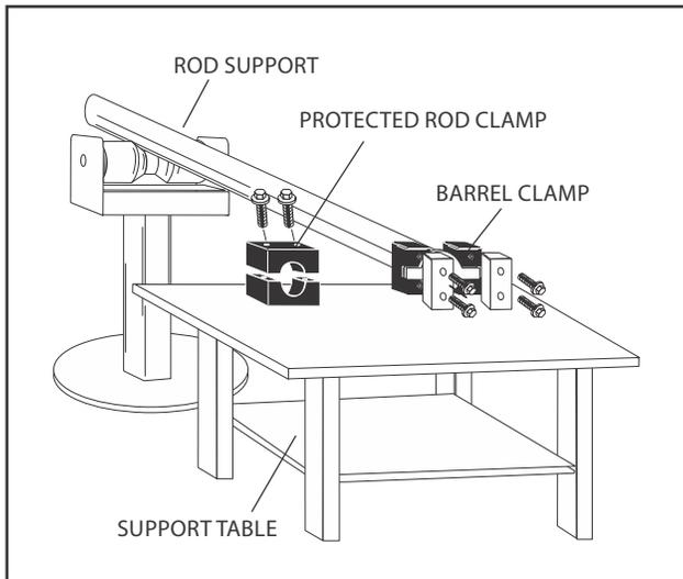
Figure 5-71. Cylinder Barrel Support
