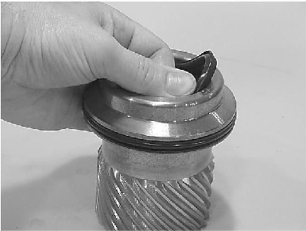
Beginning with inner seal (200) insert one end of backup ring in lower groove and feed the rest in using a circular motion. Make sure wedged ends overlap correctly.
