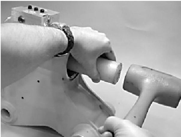
14. Remove O-ring (204) and backup ring (207) from end cap (4). Set aside for inspection.
