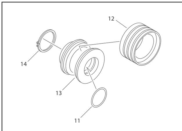
**Figure 5-26. Piston Disassembly**
