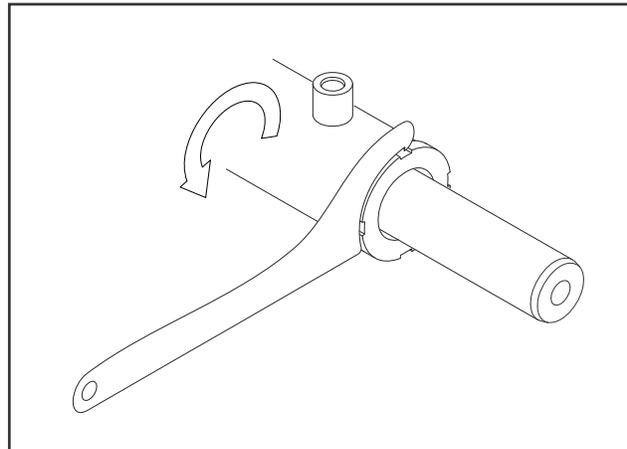
Figure 5-62. Removing Cylinder Head
