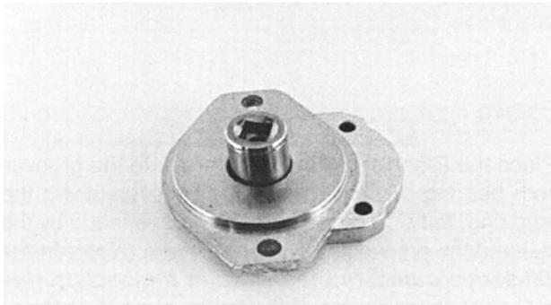
1. Install new shaft seal in mounting flange with part number side facing outboard. Press the seal into the seal bore until the seal reaches the bottom of the bore. Uniform pressure must be used to prevent misalignment or damage to the seal.
