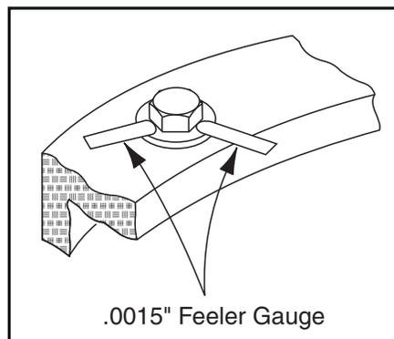
**Figure 3-50. Swing Bearing Feeler Gauge Check**
