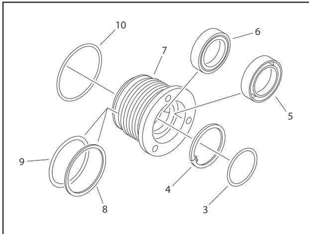
**Figure 5-29. Cylinder Head Assembly**
