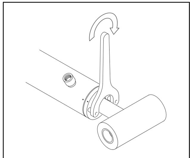
**Figure 5-31. Cylinder Head Installation**
