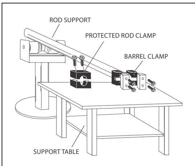
Figure 5-2. Cylinder Barrel Support
