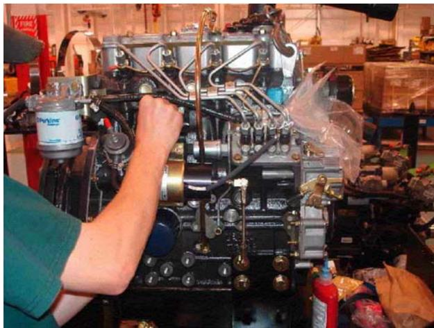
2. With control linkage pushed against idle stop, begin to make adjustments to actuator linkage to align bearing of spherical rod end with control linkage bolt hole. When making linkage adjustments, thread spherical rod end and threaded rod evenly (for every turn of spherical rod end, turn threaded rod.)
