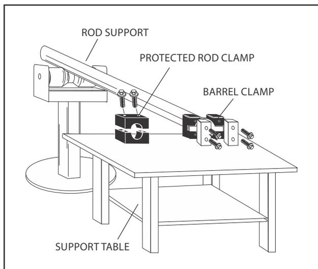
Figure 5-12. Cylinder Barrel Support
