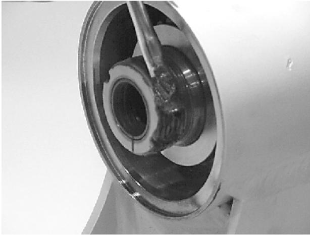
15. Install O-ring (204) and back-up ring (207) into inner seal groove on end cap (4).
