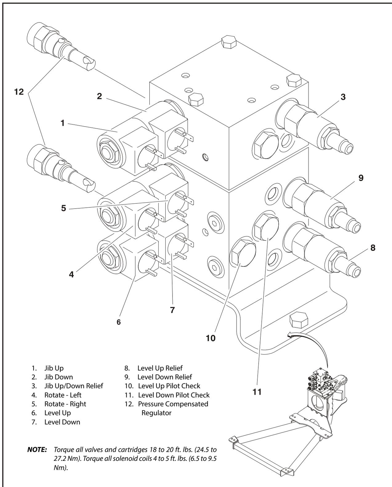
Figure 5-91. Platform Control Valve
