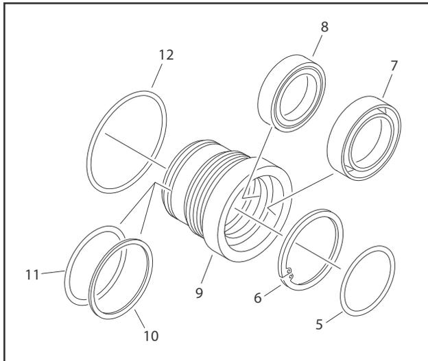
**Figure 5-78. Cylinder Head Assembly**
