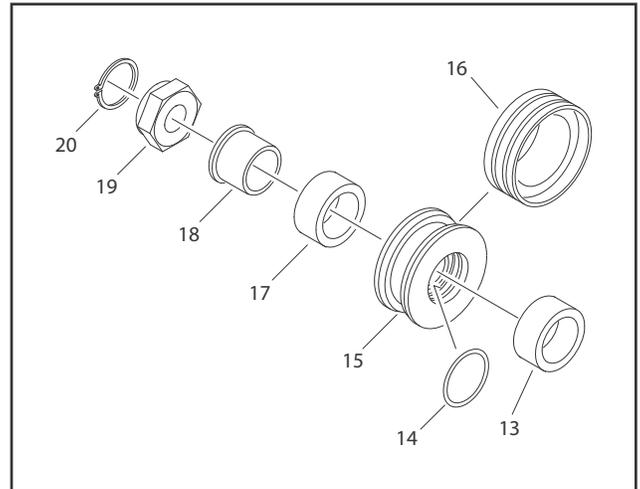
**Figure 5-59. Piston And Bushings Assembly**
