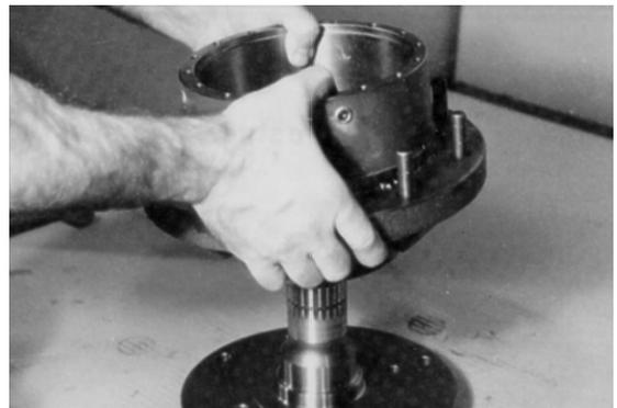
8. Press bearing cone (1F) on spindle (1A) in hub (1G).
