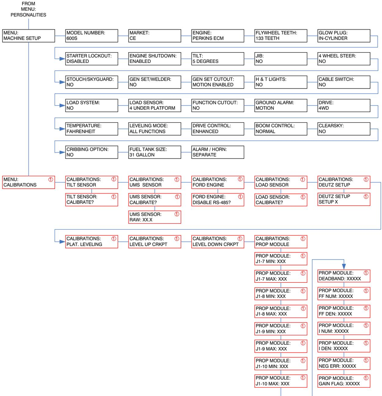
Figure 6-18. Analyzer Flow Chart, Version 6.X Software - Sheet 6 of 6
