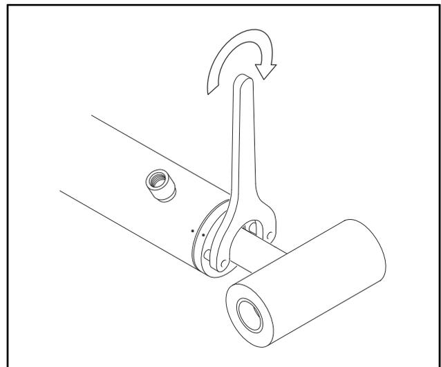
**Figure 5-50. Cylinder Head Installation**
