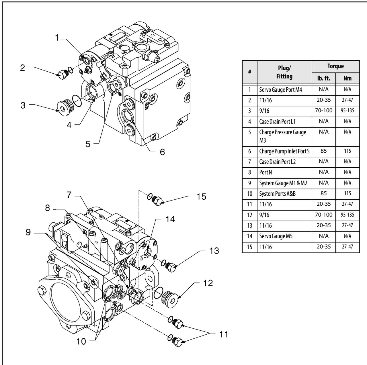
Figure 5-83. Plugs/Fittings Size & Torque
