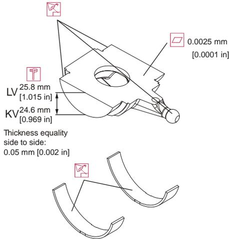
Inspect the journal bearings for damage or excessive wear. Replace journal bearings if scratched, warped, or excessively worn. The polymer wear layer must be smooth and intact.
