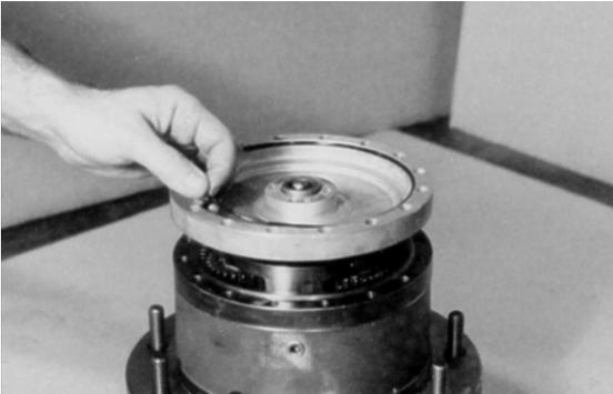
16. Place cover sub-assembly (6) on ring gear (4). Align pipe plug holes according to alignment before disassembly.
