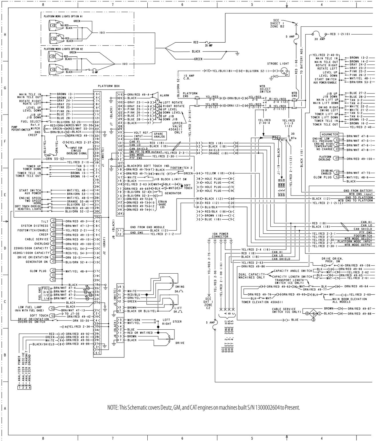
**Figure 7-30. Electrical Schematic - Deutz, GM, & CAT Engine - Sheet 1 of 4 (LH)**
