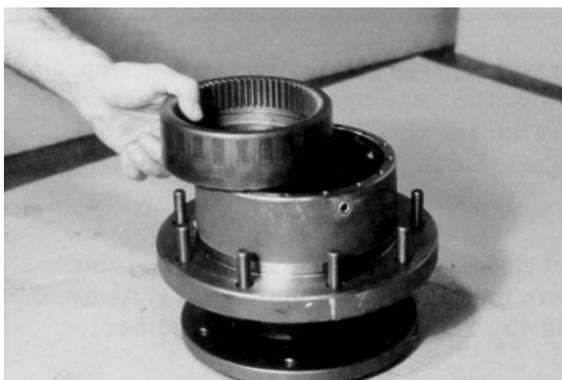
3. Place thrust washer (11) around spindle (1A) so it rests on bottom of internal gear (2).
