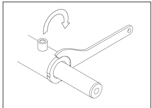
**Figure 5-80. Cylinder Head Installation**
