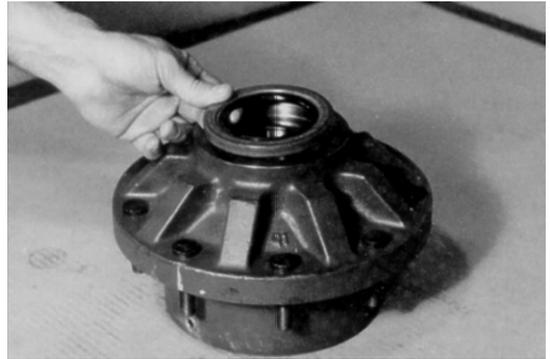
7. Oil spindle, then lower hub (1G), small end down, onto spindle (1A).
