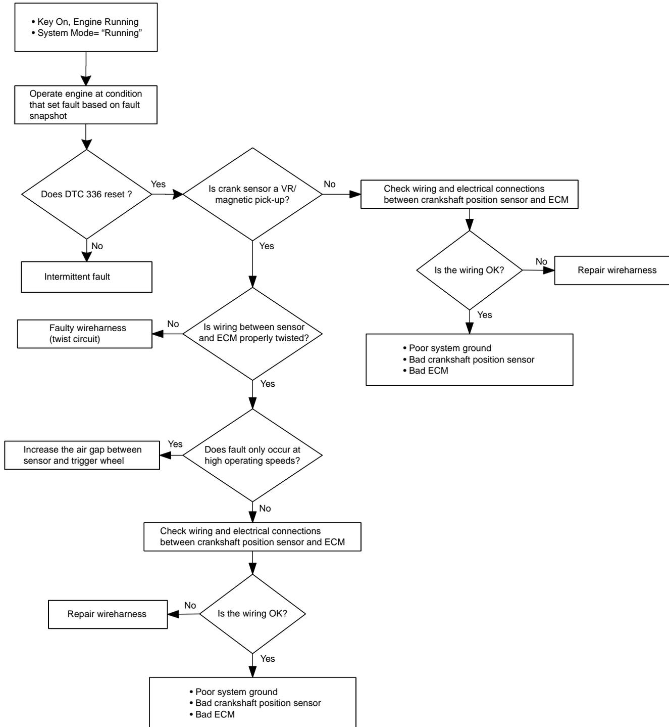
**DTC 337- Loss of Crank Input Signal**
