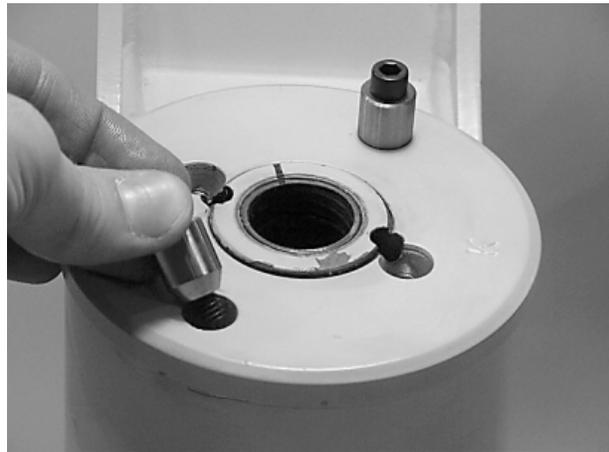
5. Using a metal bar, or something similar, unscrew end cap (4) by turning it counter clockwise.
