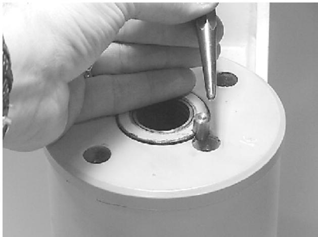
19. Insert set screws (113) over lock pins. Tighten to 25 in-lb (2.8 Nm).
