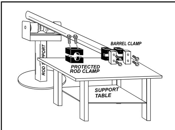
Figure 5-61. Cylinder Barrel Support
