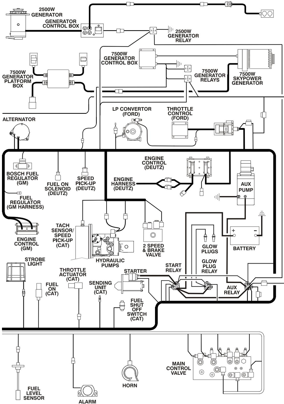
Figure 7-19. Electrical Components Installation - Sheet 2
