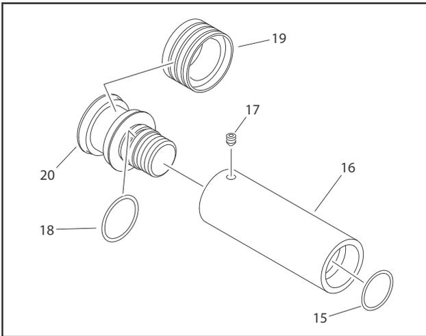
**Figure 5-36. Piston And Spacer Disassembly**
