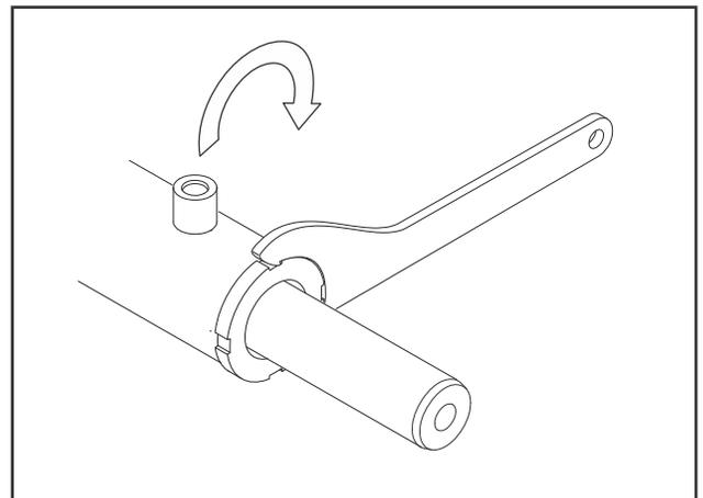
**Figure 5-69. Cylinder Head Installation**
