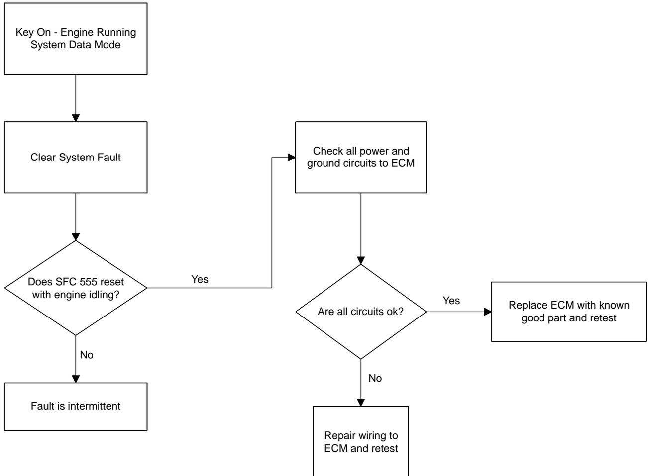
**DTC 1614- Microprocessor Failure - RTI 3**
