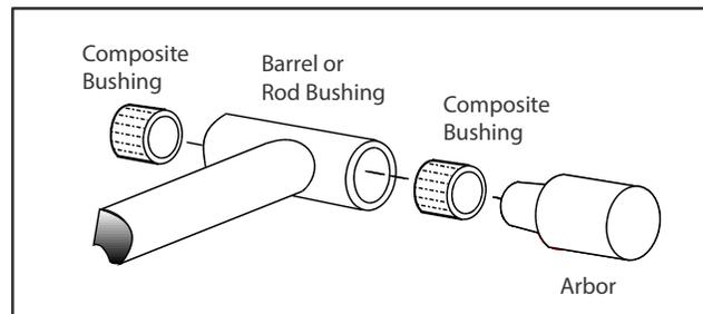
**Figure 5-47. Composite Bushing Installation**
