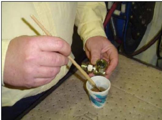
2. Hold fitting over hydraulic oil container and brush an even film of oil around entire O-ring in fitting. Make sure O-ring is completely saturated.
