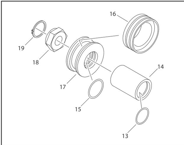
**Figure 5-6. Piston And Spacer Disassembly**
