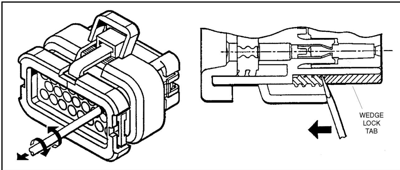
Figure 7-10. Connector Disassembly
