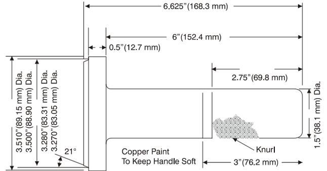
4. T-109691 ASSEMBLY PRESSING TOOL for CONE (1F)
